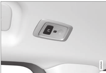
In vehicles with panoramic roofs*, there are two lamp units, one on each side of the ceiling. 7
