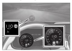
The previous illustration<sup>61</sup> shows that Adaptive Cruise Control is set to maintain a speed of 110 km/h (68 mph) and that there is no target vehicle ahead to follow.
