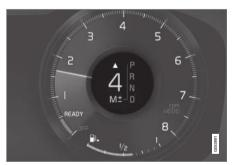
Gear indicator in 12" instrument panel\*.
