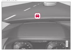
Collision warning symbol on the windshield<sup>44</sup>.
