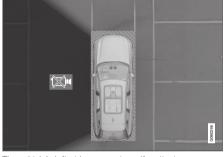
The vehicle's left-side camera is malfunctioning.
