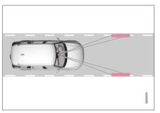
A camera monitors the traffic lane's marker lines and compares the direction of the road with the driver's movements of the steering wheel.
