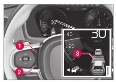
Controls for setting a time interval.
