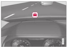
Collision warning symbol on the windshield<sup>64</sup>
