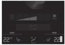
Temperature buttons in the  $\mbox{\bf Rear climate}$  tab in Climate view.
