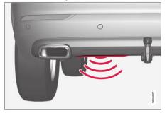
The sensor is located to the left of center under the rear bumper<sup>18</sup>.
