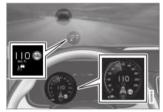
The previous illustration<sup>69</sup> shows that Pilot Assist is set to maintain a speed of 110 km/h (68 mph) and is following a target vehicle ahead that is traveling at the same speed.
