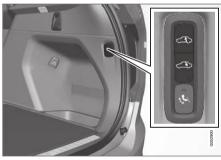
Controls for raising/lowering the rear end of the vehicle.
