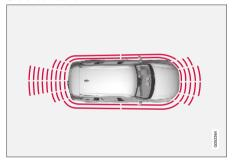
Park Assist's side sensors are automatically activated when the engine is started. They are active at speeds below 10 km/h (6 mph).
