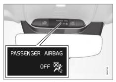
Occupant Weight Sensor (OWS) indicator light
