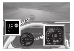
The previous illustration<sup>69</sup> shows that Pilot Assist is set to maintain a speed of 110 km/h (68 mph) and that there is no target vehicle ahead to follow.
