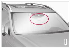
The area marked in the illustration must be kept free of decals, objects, solar film, etc.<sup>70</sup>
