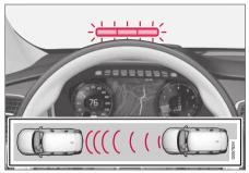
Collision warning light on the windshield<sup>43</sup>.
