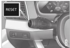
Reset all information in trip odometer TM (i.e. mileage, average fuel consumption, average speed and driving time) by pressing and holding the RESET button on the left-hand steering wheel lever.
