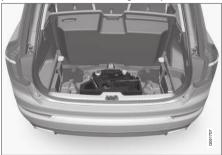
The foam block under the cargo compartment floor contains the towing eyelet, the tire sealing system, the tool for removing plastic wheel bolt covers and the tool for removing the locking wheel holts
