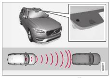
Location of the camera and radar sensor<sup>75</sup>.
