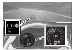
The previous illustration<sup>69</sup> shows that Pilot Assist is set to maintain a speed of 110 km/h (68 mph) and that there is no target vehicle ahead to follow.
