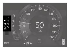
Gear indicator in 8" instrument panel.
