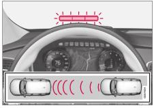
Collision warning light on the windshield<sup>63</sup>.
