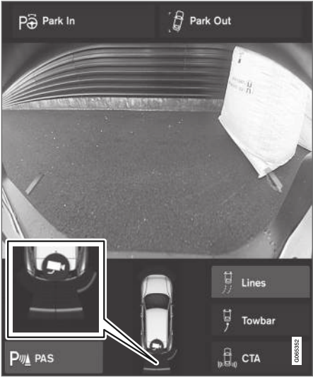
The screen can display colored sensor fields on the vehicle symbol 122 .
