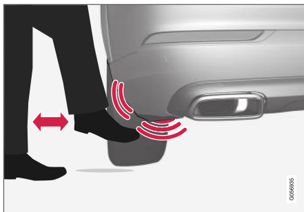
Kicking motion within the sensor's activation area.
