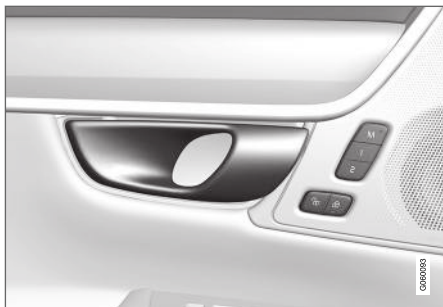
Alternative unlocking method using side door opening handle.
