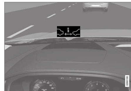
Distance Alert warning symbol on the windshield 37 .
