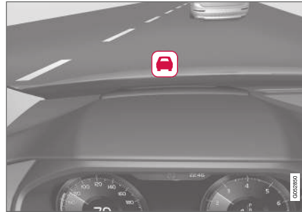
Collision warning symbol on the windshield 64 .
