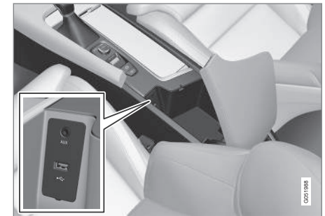
USB socket in the tunnel console
