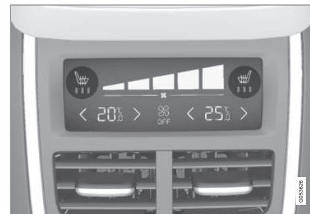
Seat heating indicator and control on the climate panel on the rear side of the tunnel console
