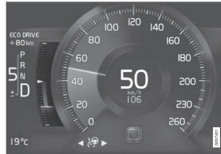
Eco gauge 8" instrument panel
