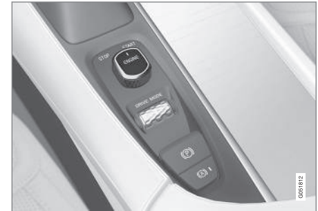
Start knob in the tunnel console
