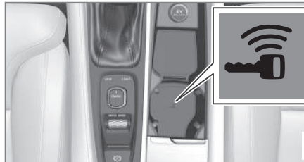
Back-up reader in the tunnel console
