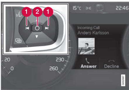
Message in the instrument panel (12" version) and the right-side steering wheel keypad
