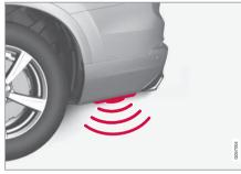
Sensor location on vehicles equipped with a skid plate/  $\operatorname{diffuser}^{\star}$
