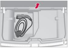
The charging cable is stowed in a storage compartment under the cargo area floor
