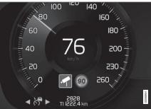
Speed camera warning in the instrument panel (generic illustration)
