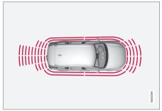
The system's side sensors are activated automatically when the engine is started and are active at speeds below approximately 6 mph (10 km/h).
