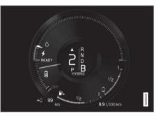
The vehicle is generating current to recharge the battery, e.g., during moderate braking or during engine braking on a downslope.
