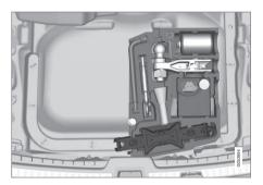
The foam block under the cargo compartment floor contains the towing eyelet, the tool for removing plastic wheel bolt covers, the jack\* and the lug wrench\*. There is also a storage space for the tool used to remove locking wheel bolts.
