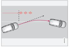
Driving lane assistance provide vibrations in the steering wheel  $\!\!\!^{8}$
