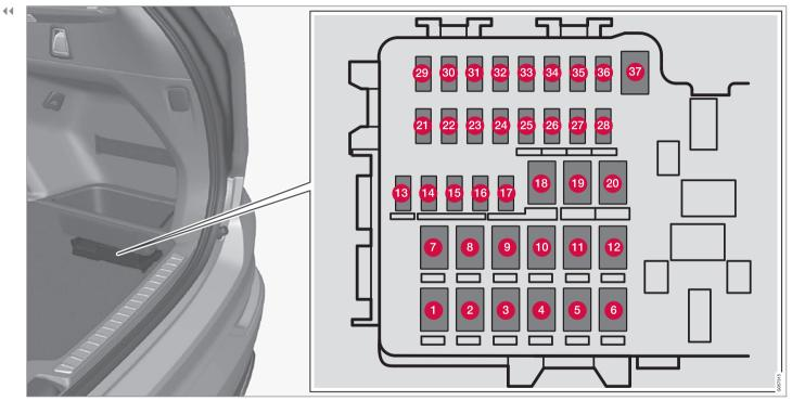
The fuse box is under the storage compartment on the right side
