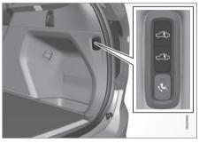
Use the buttons in the cargo compartment to raise or lower the vehicle to make loading or unloading easier or when attaching a trailer.
