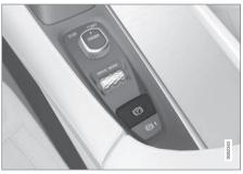
Parking brake control in the tunnel console between the front seats
