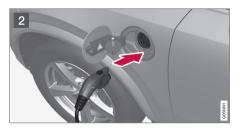
2 Open the charging door, remove the charging socket's protective cover and connect the charging cable's charge coupler.
