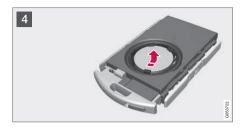
4 The battery's positive (+) side is up. Pry out the battery as shown in the illustration.
