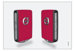
A Red Key makes it possible to limit the vehicle's maximum speed, add speed reminders and limit the audio system's volume. Several of the vehicle's safety systems will also always be active. Otherwise, this key functions in the same way as a standard remote key.
