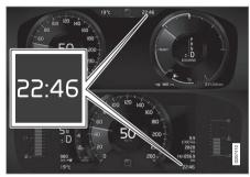
Location of the clock in the instrument panel in 12" (upper) and 8" (lower) instrument panels
