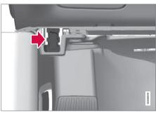
The diagnostic socket OBDII under the dashboard on the driver's side
