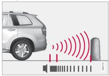
The system's rear sensors are activated automatically when the engine is started and are active if the vehicle rolls rearward with the gear selector in  $\mathbf{N}$  or if  $\mathbf{R}$  has been selected.
