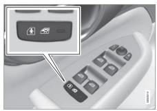
Child safety lock button on the driver door control panel
