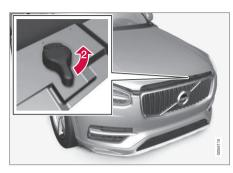
Turn the handle under the front edge of the hood counterclockwise to release it from the lock and lift.
