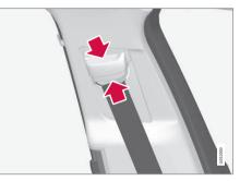
Press the button and move the upper seat belt anchor up or down.
