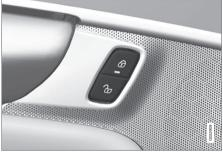
Central locking/unlocking buttons and indicator lights on the front doors
