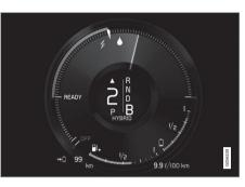
The electric motor alone cannot provide the power requested and the gasoline engine will start.
