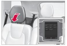
The outboard head restraints can be folded down in two ways from the center display.
