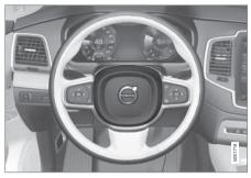
The horn is located in the steering wheel hub.
