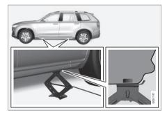
Raise the vehicle until the wheel to be changed is lifted off the ground. Remove the wheel bolts.
