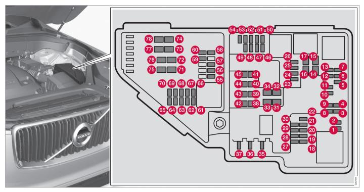
There is a fuse removal tool on the inside of the fuse box cover. There are also positions in the fuse box for several extra fuses.
