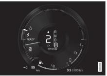
Current is generated to charge the hybrid battery, such as light braking and when engine braking on downslopes
