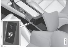
AUX/USB sockets in the tunnel console
