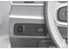
The intensity of the mood lighting can also be fine-tuned using the thumb wheel (on the dashboard to the left of the steering wheel)
