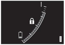
The "Hold" or "Charge" function is activated, which is shown by the ft symbol near the battery indicator. See also the article "Maintaining/ increasing hybrid battery charge while driving" for additional information.
