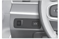
The ambience lighting can also be fine-tuned using the thumb wheel (on the dashboard to the left of the steering wheel)
