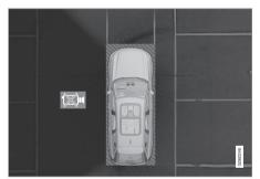
In this example, the driver's side camera is not function-
