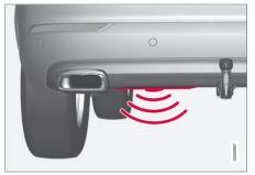
The foot movement sensor is located to the left of center under the rear  ${\rm bumper}^6$
