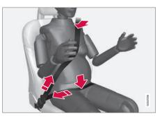
The diagonal section should wrap over the shoulder then be routed between the breasts and to the side of the belly. The lap section should lay flat over the thighs and as low as possible under the belly. It must never be allowed to ride upward. Remove all slack from the belt and ensure that it fits close to the body without any twists.
