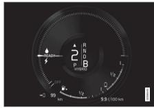
The vehicle has started but is stationary and no power is being utilized.
