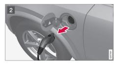
Press the release button on the charge coupler to release it and disconnect the coupler from the vehicle's charging socket. Remove the cable from the vehicle. Put the socket's cover back in place and close the charger door.
