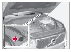
The windshield and headlight washers\* share a common reservoir. Open the blue cap to refill washer fluid (see the illustration for the location of the reservoir).
