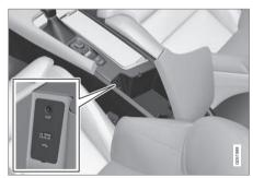
USB socket in the tunnel console
