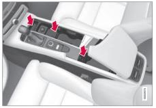
Storage spaces, cup holders and 12-volt socket/AUX/USB sockets in the tunnel console in the tunnel console
