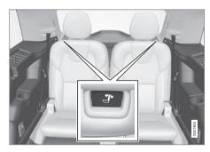
1. Pull the handle on the upper side of the backrest upward/forward.
