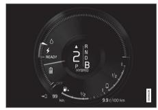
Battery charging gauge in the instrument panel
