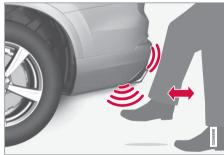
Kicking motion under the sensor's activation area
