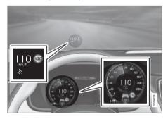
In this illustration, Pilot Assist is set at 65 mph (110 km/h) and there is no target vehicle ahead.
