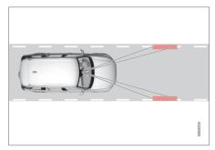
A camera monitors the traffic lane's side marker lines and compares the direction of the road with the driver's movements of the steering wheel.
