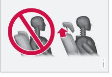
The center head restraint should be adjusted up or down according to the passenger's height. The restraint should be carefully adjusted to support the occupant's head.
