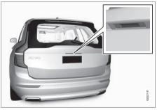
Rubberized button on the tailgate used only for unlocking
