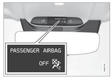
Occupant Weight Sensor (OWS) indicator light
