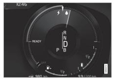
The instrument panel gauge when both the electric motor and gasoline engine are being used
