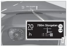
The head up-display presents types of information that the driver should be aware of immediately, such as traffic warnings, speed information and navigation. Road sign information and incoming phone calls are also displayed here. The head-up display is controlled from the right-side steering wheel keypad and the center display.
