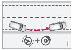
Run-off Mitigation provides steering assistance and braking
