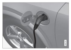
Place the charging socket's protective cover on the holder provided on the charging socket door. 4. The charging cable's coupler will lock onto the charging socket and charging will begin within approx. 10 seconds. The approximate remaining charging time and charging status will be displayed in the instrument panel. See also the article "Hybrid battery charge status."
