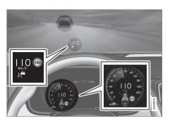
In this illustration, Pilot Assist is set at 65 mph (110 km/h) and there is a target vehicle ahead that is traveling at the same speed.
