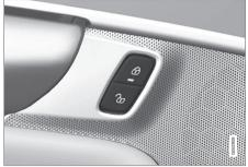
Front door lock button and indicator light Indicator lights on: all doors are locked.
