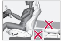
Do not place any objects behind the front seats that could impede the WHIPS function
