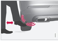
Kicking motion under the sensor's activation area
