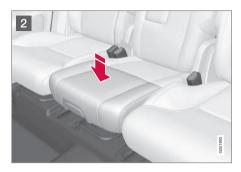
2 Press down on the center of the booster cushion to return it to the stowed position.
