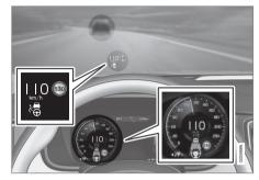
In this illustration, Pilot Assist is set at 65 mph (110 km/h) and there is a target vehicle ahead that is traveling at the same speed.
