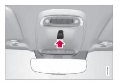
The laminated panoramic roof and the sun shade are operated using the controls in the ceiling console, near the rear-view mirror. The controls are activated when the vehicle's ignition is in mode I or II.
