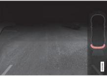
The screen can display colored sensor fields on the car symbol at the right
