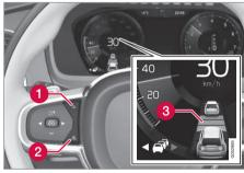
Controls for setting a time interval
