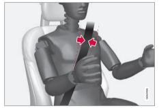
The seat belt should be positioned over the shoulder (not over the arm)
