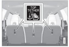
Top tether anchors and symbols on the rear side of the second row backrests. There is no symbol for the center anchor position.
