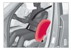
The SIPS airbag system is designed to help increase occupant protection in the event of certain side impact collisions. The SIPS airbags are designed to deploy only during certain sideimpact collisions, depending on the crash severity, angle, speed and point of impact.
