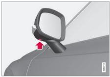
The side cameras are located in the respective door mirrors and shows views along the sides of the vehicle.
