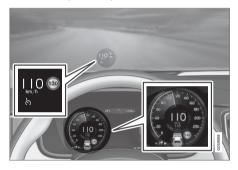
This illustration<sup>4</sup> shows that ACC is set at a speed of 68 mph (110/km/h) and that there is no vehicle ahead to follow.
