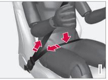
The lap section of the belt must be positioned low on the hips (not pressing against the abdomen)
