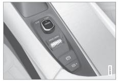
Start knob in the tunnel console between the front seats
