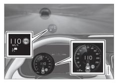
This illustration<sup>4</sup> shows that ACC is set at a speed of 68 mph (110/km/h) and is following another vehicle traveling at the same speed.
