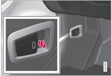
With the hood completely closed, pull the control (located to the left of the brake pedal).
