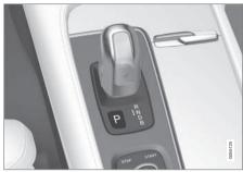
Park is activated using a switch located next to the gear selector.
