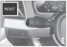
Reset trip odometer TM by pressing and holding the **RESET** button the left-side steering wheel lever. Trip odometer TA resets automatically if the ignition is switched off for more than 4 hours.
