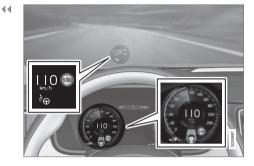
In this illustration, Pilot Assist is set at 65 mph (110 km/h) and there is no target vehicle ahead.
