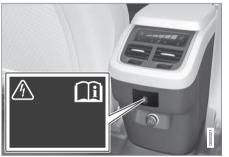
120-volt socket in the tunnel console for the second row of seats
