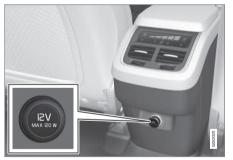
12-volt socket in the tunnel console for the second row of seats
