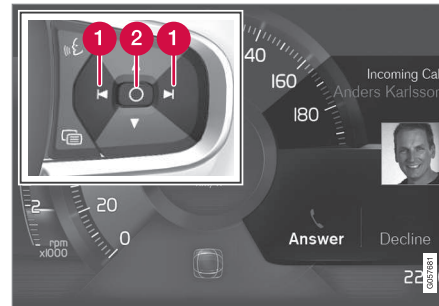
Message in the instrument panel (8" version) and the right-side steering wheel keypad
