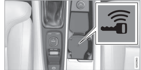
Back-up reader in the tunnel console
