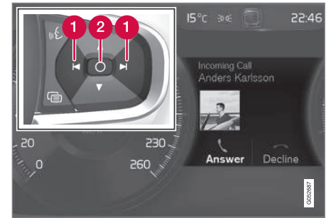
Message in the instrument panel (12" version) and the right-side steering wheel keypad
