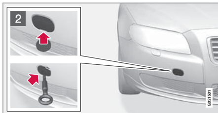
Attaching the towing eyelet
