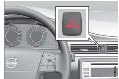
Location of the hazard warning flasher button
