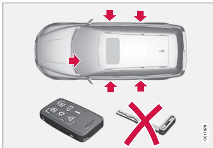
Locking/unlocking points with private locking activated.
