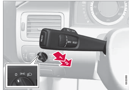
Headlight switch and lever
