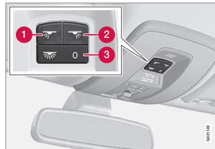
Light switches, front roof lighting
