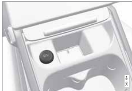
12-volt socket in the front tunnel console
