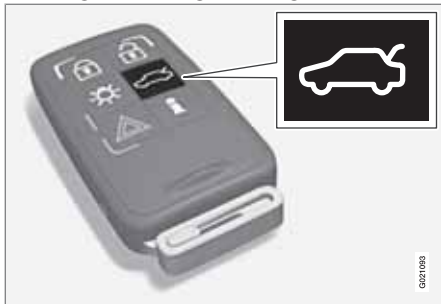
Tailgate unlock button on the remote key
