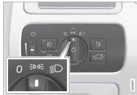
Headlight control in position for parking lights
