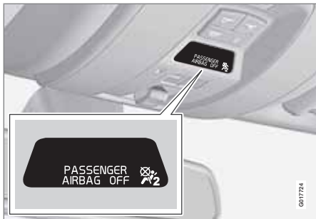
Occupant Weight Sensor (OWS) indicator light
