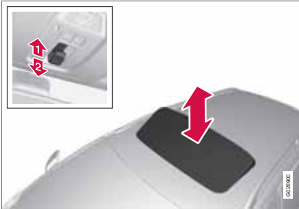
Tilt position, raised at the rear edge
