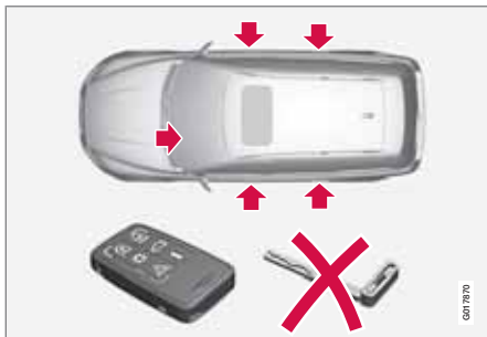
Locking/unlocking points with private locking activated.
