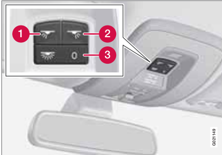
Light switches, front roof lighting
