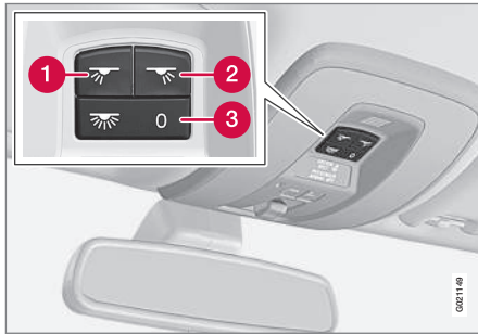
Light switches, front roof lighting
