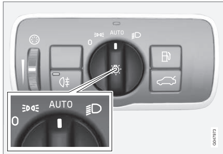
Headlight switch in the AUTO position
