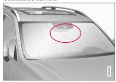
The area marked in the illustration must be kept free of decals, objects, solar film, etc.<sup>63</sup>
