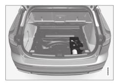
The foam block under the cargo compartment floor contains the towing eyelet, the tire sealing system, the tool for removing plastic wheel bolt covers and the tool for removing the locking wheel bolts.
