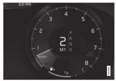
Manual shifting mode in the instrument panel<sup>2</sup>.
