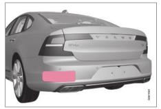
Keep the marked area clean (on both the left and right sides of the vehicle)86.
