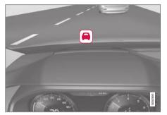
Collision warning symbol on the windshield<sup>39</sup>.
