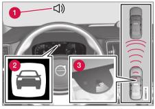
Collision warning audible signal and symbol<sup>56</sup>.
