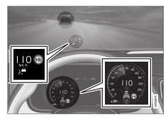
The previous illustration  $^{62}$  shows that Pilot Assist is set to maintain a speed of 110 km/h (68 mph) and is following a target vehicle ahead that is traveling at the same speed.
