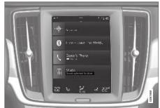
Many of the vehicle's main functions are controlled from the center display, a touchscreen that reacts to taps and other gestures. This minimizes the number of physical buttons and controls needed in the vehicle. The screen can also be operated while wearing gloves.
