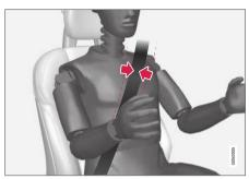
The belt should be positioned closely over the shoulder (against the collarbone, not down over the arm).
