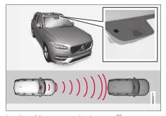
Location of the camera and radar sensor<sup>68</sup>.
