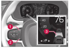
Controls for setting a time interval<sup>43</sup>.
