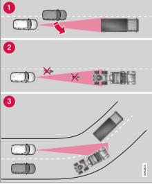
The radar sensor's field of vision.
