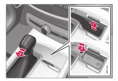
If the vehicle cannot be driven (e.g. due to a discharged battery), the gear selector must be moved to the  ${\bf N}$  position so that the vehicle can be moved.
