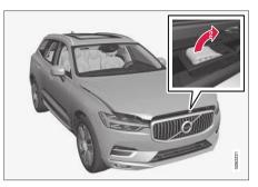
Swipe your hand from left to right under the hood, grasp the handle and move it up and to the side to release the catch and lift the hood.
