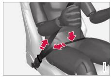
The lap section of the seat belt should be positioned low on the hips (not against the abdomen).
