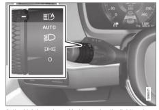
Active high beam is enabled by moving the lighting ring on the steering wheel lever to  $\,$  AUTO  $\,$  .
