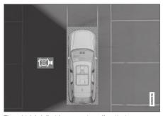
The vehicle's left-side camera is malfunctioning.
