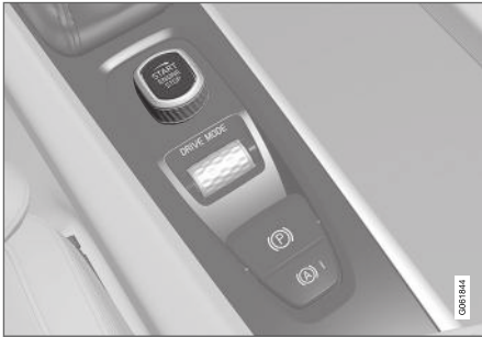
Start knob in the tunnel console.
