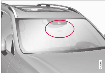
The area marked in the illustration must be cleaned regularly and kept free of decals, objects, solar film, etc.
