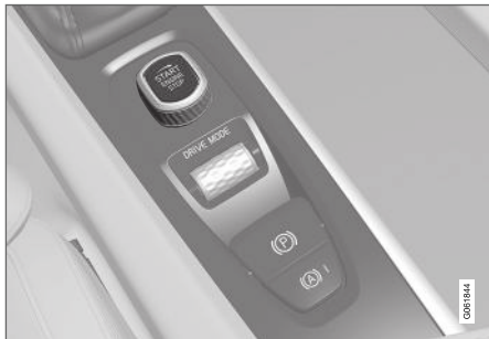
Start knob in the tunnel console.
