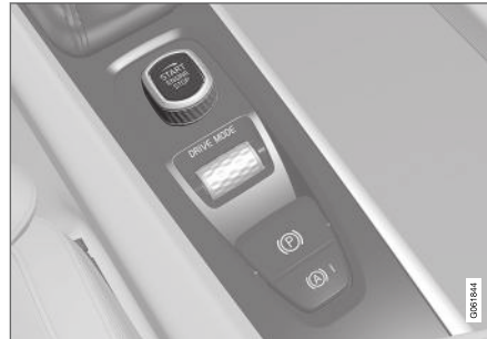
Start knob in the tunnel console.
