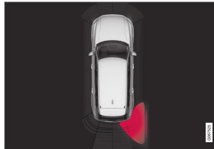
Illuminated CTA icon in the Park Assist System graphic on the screen.
