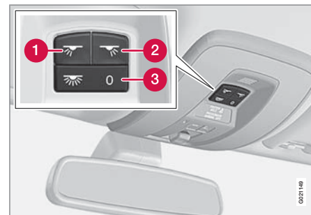
Light switches, front roof lighting
