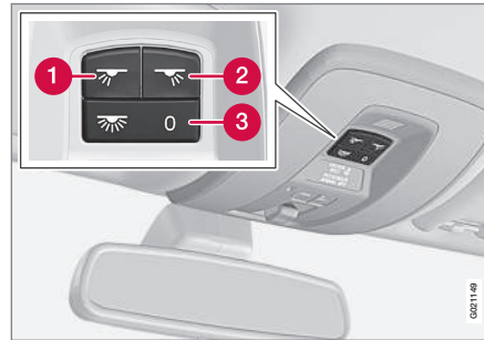
Light switches, front roof lighting
