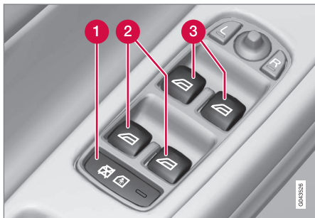
Driver's door control panel
