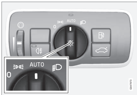
Headlight switch in the AUTO position
