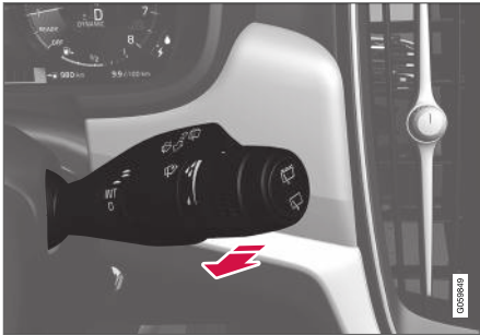
Washing function, right-hand steering wheel lever.
