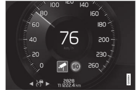
Speed camera information in the instrument panel 98 .
