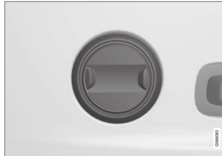
Control in vehicles with two-way lumbar support*.
