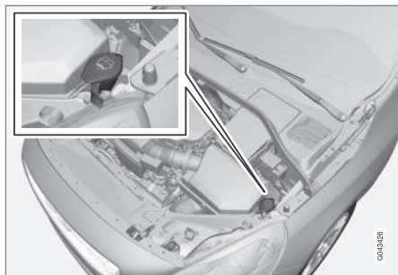
Location of the washer fluid reservoir
