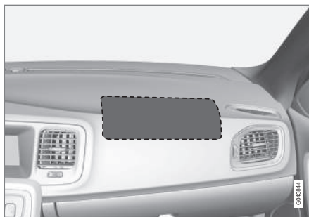
Location of the passenger's side front airbag
