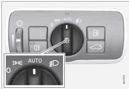
Headlight switch in the AUTO position
