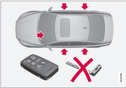
Locking/unlocking points with valet locking activated
