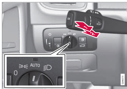
Headlight switch and steering wheel lever
