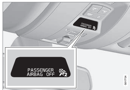
Occupant Weight Sensor (OWS) indicator light
