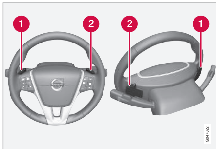
Steering-wheel mounted gear shift paddles
