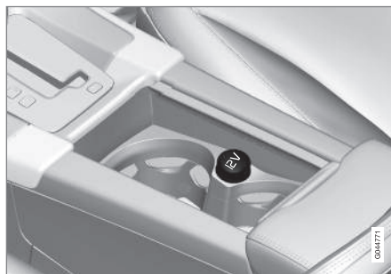
12-volt socket in the front tunnel console
