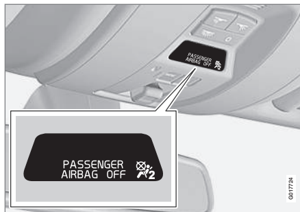
Occupant Weight Sensor (OWS) indicator light
