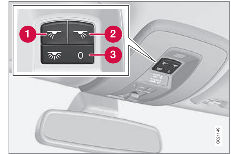
Light switches, front roof lighting
