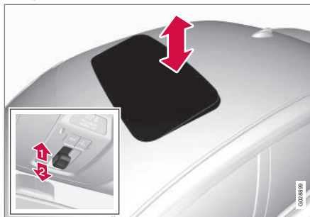
Tilt position, raised at the rear edge
