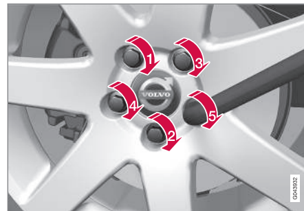
Tighten the wheel nuts
