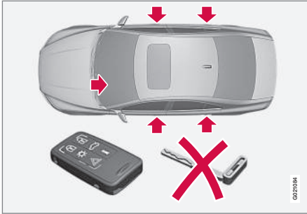
Locking/unlocking points with valet locking activated
