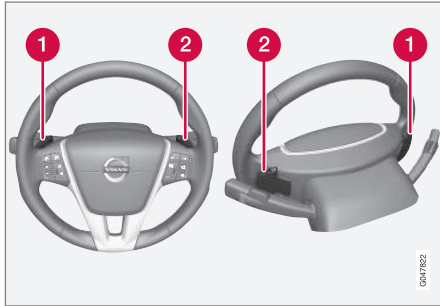
Steering-wheel mounted gear shift paddles
