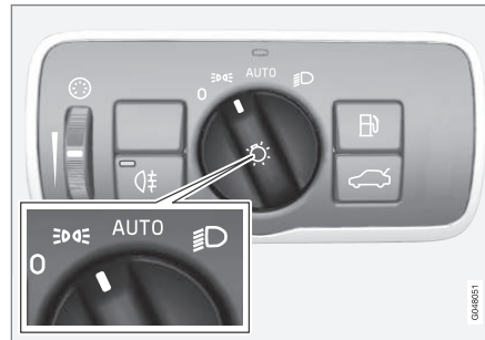
Headlight switch in the parking light position
