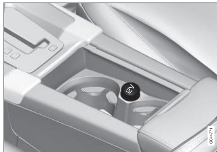
12-volt socket in the front tunnel console
