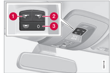
Light switches, front roof lighting
