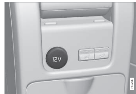
12-volt socket in the rear center console
