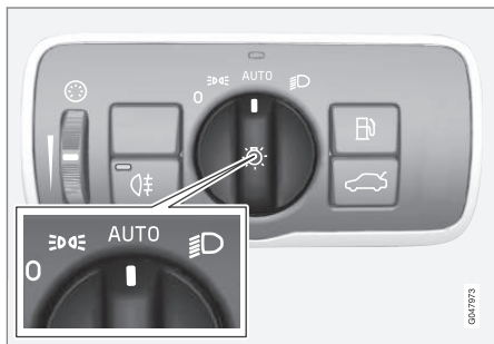
Headlight switch in the AUTO position
