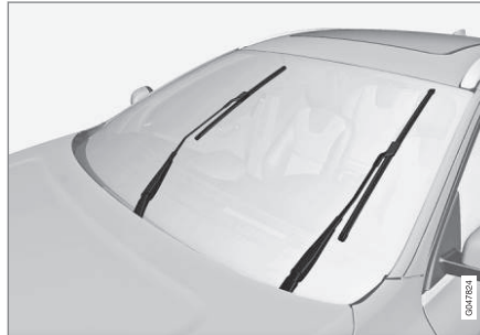
Wiper blades in service position
