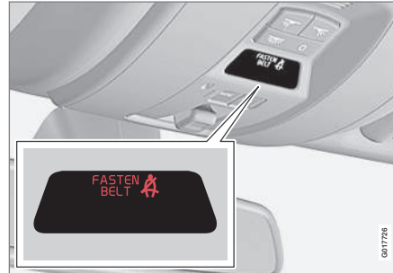
Seat belt reminder light in ceiling console
