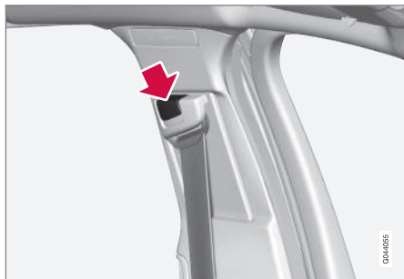
Adjusting seat belt height
