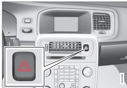
Location of the hazard warning flasher button
