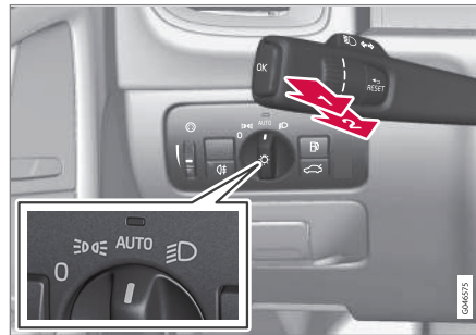
Headlight switch and steering wheel lever
