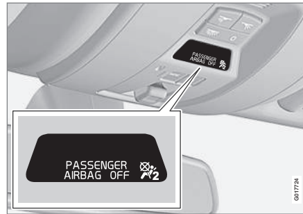
Occupant Weight Sensor (OWS) indicator light
