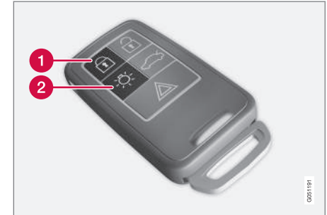
Remote key buttons used for remote engine start
