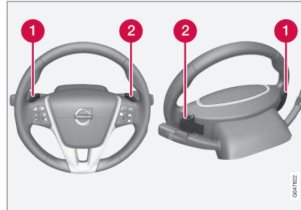
Steering-wheel mounted gear shift paddles
