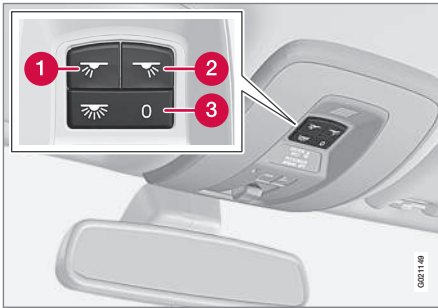
Light switches, front roof lighting
