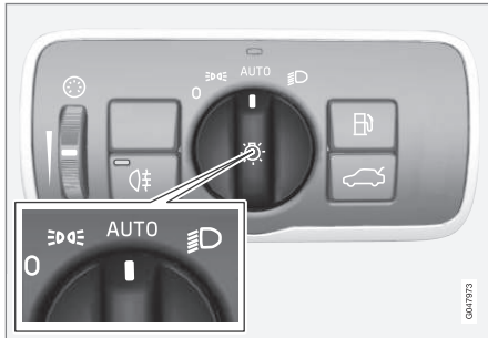
Headlight switch in the AUTO position
