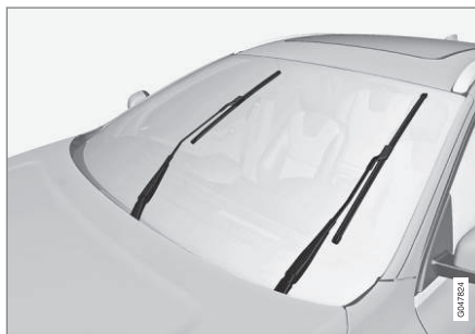
Wiper blades in service position
