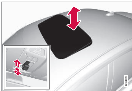
Tilt position, raised at the rear edge
