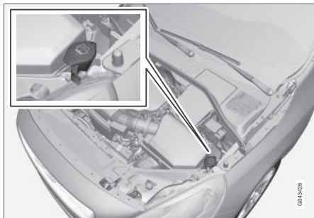
Location of the washer fluid reservoir
