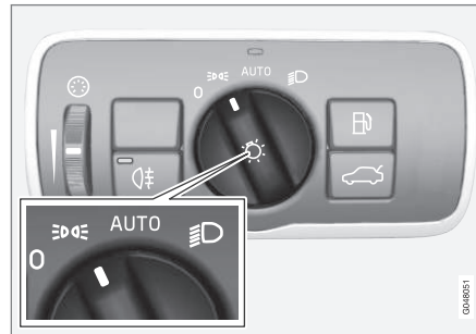
Headlight switch in the parking light position
