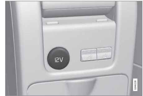
12-volt socket in the rear center console
