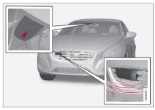
Camera and radar sensor<sup>6</sup>.
