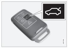
Tailgate unlock button on the remote key
