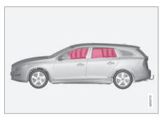
This system consists of inflatable curtains located along the sides of the roof liners, stretching from the center of both front side windows to the rear edge of the rear side door windows.
