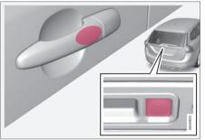
Models with keyless drive have a pressure-sensitive area on the outside door handles and a rubber-covered button next to the tailgate opening control
