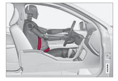
The diagonal section should wrap over the shoulder then be routed between the breasts and to the side of the belly. The lap section should lay flat over the thighs and as low as possible under the belly. It must never be allowed to ride upward. Remove all slack from the belt and ensure that it fits close to the body without any twists.
