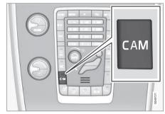
PAC is activated when the gear selector is moved to **R** if the system is selected in the **MY CAR** menu system or by pressing the **CAM** button in the center console. See My Car – introduction (p. 77) for a description of the menu system.
