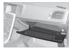
The owner's manual and maps can be kept here. There are also holders for pens and fuel cards. The glove compartment can be locked manually with the key blade, see Locking/unlocking glove compartment (p. 166).
