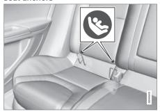
Symbols on the seat back upholstery mark the ISOFIX/LATCH anchor positions as shown. To access the anchors, kneel on the seat cushion and locate the anchors by feel. Always follow your child seat manufacturer's installation instructions, and use both ISOFIX/LATCH lower anchors and top tethers (p. 58) whenever possible.
