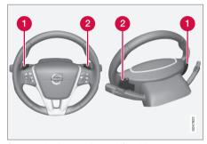
Steering-wheel mounted gear shift paddles
