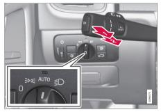
Headlight switch and steering wheel lever
