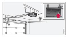
At the garage door opener receiver (motorhead unit) in the garage, locate the "learn" or "smart" button. This can usually be found where the hanging antenna wire is attached to the motor-head unit.
