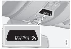
Occupant Weight Sensor (OWS) indicator light
