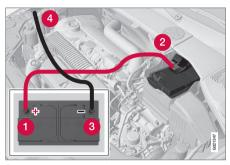
Connecting the jumper cables
