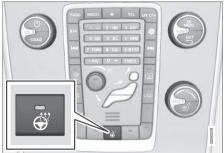
Button for steering wheel heating
