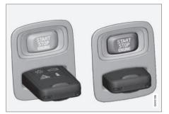
Ignition slot with remote key inserted (see Ignition modes (p. 80) for more information on ignition modes)
