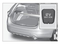
Fold down the cover to access the electrical socket.
