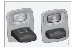
To turn off the alarm, insert the remote key into the ignition slot (also on vehicles with the optional keyless drive). 3. Start the engine.
