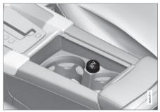
12-volt socket in the front tunnel console
