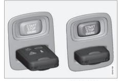
Ignition slot with remote key and START/STOP **ENGINE** button.
