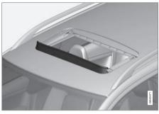
The moonroof is equipped with a wind blocker that folds up when the moonroof is open.
