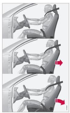
In the event of a rear-end collision, the hinges and brackets of the front seat backrests are designed to change position slightly to allow the backrest/head restraint to help support the occupant's head before moving slightly rearward. This movement helps absorb some of the forces that could result in whiplash.
