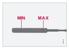
The oil level must be between the  ${\bf MIN}$  and  ${\bf MAX}$  marks on the dipstick
