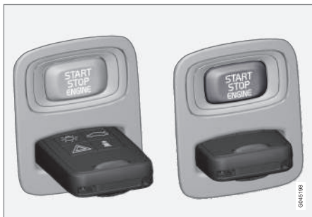
Ignition slot with remote key inserted (see Ignition modes (p. 74) for more information on ignition modes)
