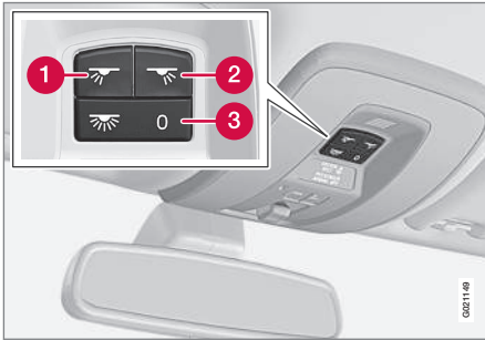
Light switches, front roof lighting
