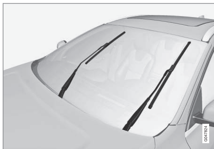
Wiper blades in service position
