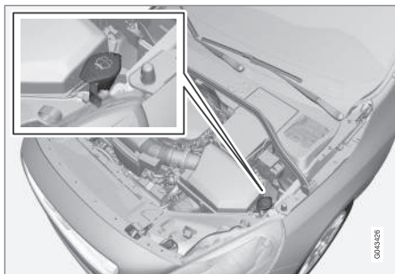
Location of the washer fluid reservoir
