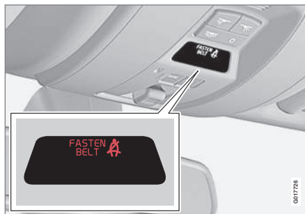
Seat belt reminder light in ceiling console
