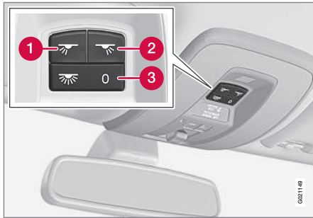
Light switches, front roof lighting
