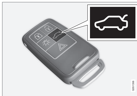
Tailgate unlock button on the remote key
