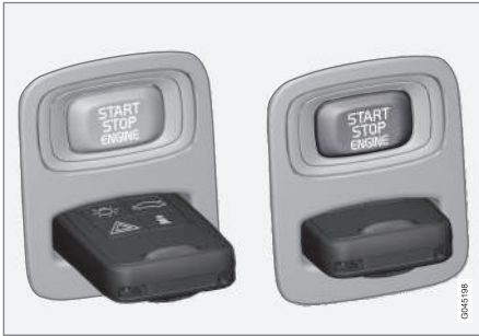
Ignition slot with remote key inserted (see Ignition modes (p. 82) for more information on ignition modes)
