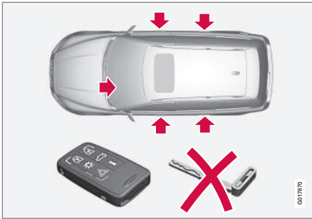
Locking/unlocking points with private locking activated.
