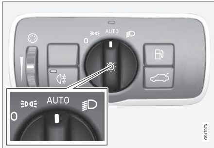
Headlight switch in the AUTO position
