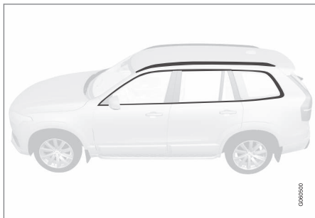
Components that should be washed with a cleaning product with a pH value between 3.5 till 11.5 (generic illustration)
