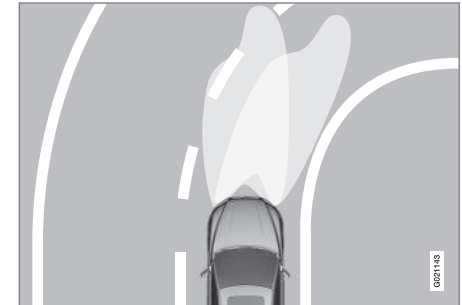
Headlight pattern with the Active Bending Light function deactivated (left) and activated (right)
