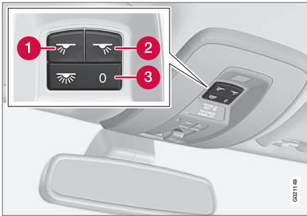
Light switches, front roof lighting
