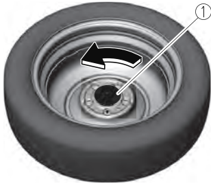
1. Spare tire hold-down bolt
