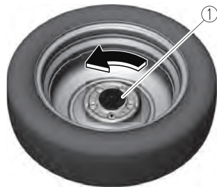
1. Spare tire hold-down bolt
