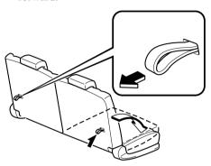
5. Lock the seatback in place by pushing it down. Make sure the seatback is secured by attempting to lightly move it up and down.
