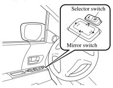
After adjusting the mirror, lock the control by placing the selector switch in the center position.
