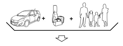
GCW (Gross Combination Weight) is the weight of the loaded vehicle (GVW).
