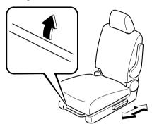
Make sure the lever returns to its original position and the seat is locked in place by attempting to push it forward and backward.
