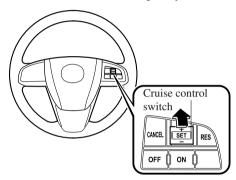
Your vehicle has a tap-up feature that allows you to increase your current speed in increments of 1.6 km/h (1 mph) by a momentary tap of the cruise control SET + switch. Multiple taps will increase your vehicle speed 1.6 km/h (1 mph) for each tap.
