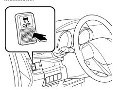
Press the switch again to turn the TCS/DSC back on. The DSC OFF indicator light turns off.
