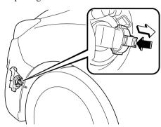
4. Turn the bulb assembly counterclockwise and remove it. Carefully remove the bulb from its socket in the reflector by gently pulling it straight backward out of the socket.
