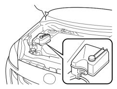
If it is at or near L, add enough coolant to the coolant reservoir to provide freezing and corrosion protection and to bring the level to F.
