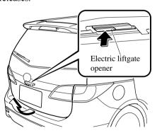
While the ignition is switched ON, the liftgate can be opened only when the vehicle is stopped with the parking brake applied (manual transaxle), or with the selector lever in the P position (automatic transaxle).
