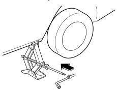
7. Turn the lug wrench clockwise and raise the vehicle high enough so that the spare tire can be installed. Before removing the lug nuts, make sure your Mazda is firmly in position and that it cannot slip or move.
