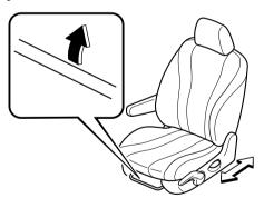
Make sure the lever returns to its original position and the seat is locked in place by attempting to push it forward and backward.
