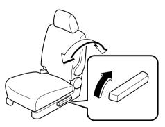
Make sure the lever returns to its original position and the seatback is locked in place by attempting to push it forward and backward.
