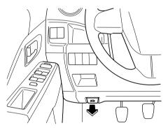
Insert your hand into the hood opening, slide the hood latch lever, and lift the hood.
