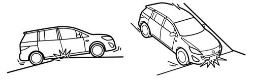
Your vehicle is equipped with low profile tires allowing class-leading performance and handling. As a result, the sidewall of the tires are very thin and the tires and wheels can be damaged if driven through potholes or on rough/uneven roads at excessive speeds. Use care and reduce speed when traveling on rough/uneven roads or through potholes.
