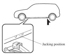
5. Continue raising the jack head gradually by rotating the screw with your hand until the jack head is inserted into the jack-up position.
