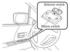
After adjusting the mirror, lock the control by placing the selector switch in the center position.
