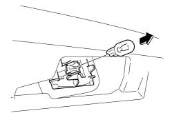
4. Install the new bulb in the reverse order of the removal procedure.
