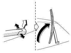
Firmly rotate the wiper blade to the right until it unlocks, then remove the blade.
