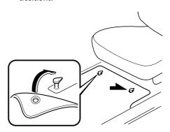
When setting a floor mat, position the floor mat so that its eyelets are inserted over the pointed end of the retention posts.
