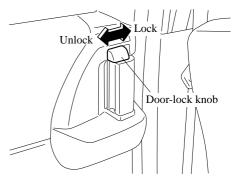
To lock a sliding door with the door-lock knob from the outside, slide the door-lock knob toward the front to the lock position and close the door (pulling the door handle is not required).
