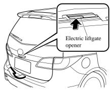
While the ignition is switched ON, the liftgate can be opened only when the vehicle is stopped with the parking brake applied (manual transaxle), or with the selector lever in the P position (automatic transaxle).
