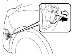
Turn the bulb assembly counterclockwise and remove it. Carefully remove the bulb from its socket in the reflector by gently pulling it straight backward out of the socket.
