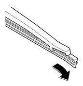
4. Remove the metal stiffeners from each blade rubber and install them in the new blade.
