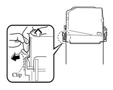
3 Pull out the battery cover being careful not to allow it to contact the cowl grille.
