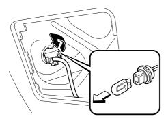
5. Install the new bulb in the reverse order of the removal procedure.
