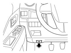
Insert your hand into the hood opening, slide the hood latch lever, and lift the hood.
