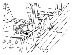
4. Disconnect the electrical connector from the bulb by pressing the tab on the connector with your finger and pulling the connector.
