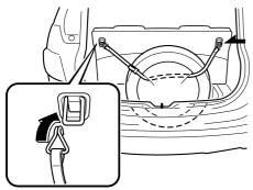
11. Pull the belt end to secure the flat tire.
