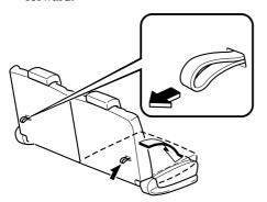
5. Lock the seatback in place by pushing it down. Make sure the seatback is secured by attempting to lightly move it up and down.
