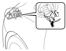
Turn the bulb assembly counterclockwise and remove it.
