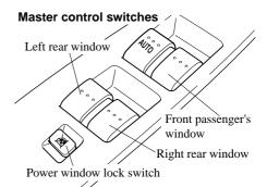
To open the window to the desired position, hold down the switch. To close the window to the desired position, pull up the switch.
