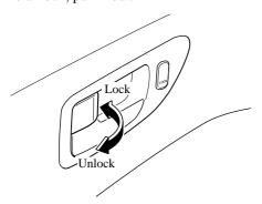
To lock either front door with the door-lock knob from the outside, push the door-lock knob to the lock position and close the door (pulling the door handle is not required).
