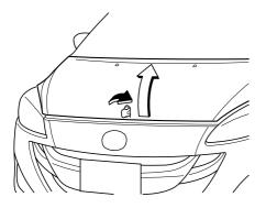
Grasp the support rod in the padded area and secure it in the support rod hole indicated by the arrow to hold the hood open.
