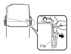
2 Detach the clip facing the vehicle interior first and pull it outward with your finger approx. 4 mm (0.2 in). Then, lift the cover slightly to clear the lock.
