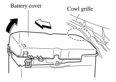
**Installing battery cover**
