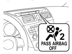
If the front passenger weight sensors are normal, the indicator light illuminates when the ignition is switched ON. The light turns off after a few seconds.
