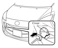
3. Securely install the tiedown eyelet using the lug wrench.
