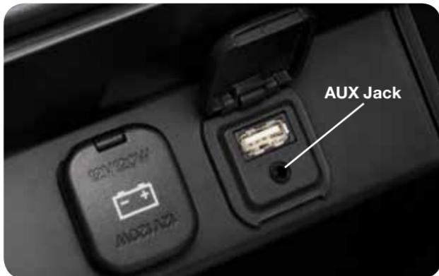
**NOTE:** You will need an audio cable with an 1/8 inch (3.5 mm) mini stereo plug (available as a Genuine Mazda accessory) to connect your portable audio player into the AUX jack.
