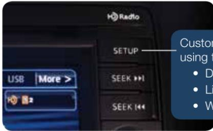
Customize the following vehicle functions using the audio SETUP button:
