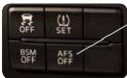
Push AFS OFF to turn system off or on. When off, AFS OFF illuminates in the instrument panel.
