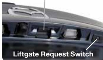
**NOTE:** When the liftgate opener switch is pushed, the liftgate will open slightly. If the liftgate is not opened within 1.5 seconds, the liftgate latch locks (you will hear it lock) and the liftgate cannot be opened or closed from this slightly raised position. To open/close the liftgate, push the liftgate opener switch, open the liftgate within 1.5 seconds, then close it. The door/liftgate ajar warning light will be on if the liftgate is not fully closed.
