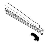
3. Remove the metal stiffeners from each blade rubber and install them in the new blade.
