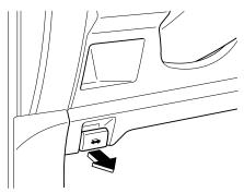
2. Insert your hand into the hood opening and slide the hood latch to the right and lift the hood.
