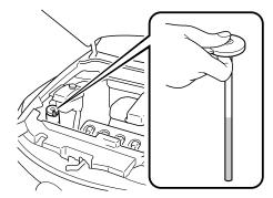
To inspect the washer fluid level in the front reservoir, pull off the cap. Then, holding your thumb over the hole in the center of the cap, lift it straight up. The fluid level can be seen from the fluid column in the pipe. Add fluid if necessary.
