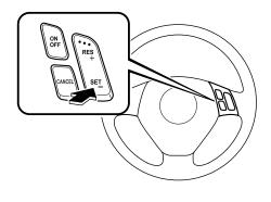
Your vehicle has a tap-down feature that allows you to decrease your current speed in decrements of 1.6 km/h (1 mph) by a momentary tap of the SET/- button. Multiple taps will decrease your vehicle speed 1.6 km/h (1 mph) for each tap.
