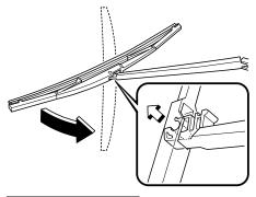
To prevent damage to the rear window let the wiper arm down easily, don't let it slap down on the rear window.
