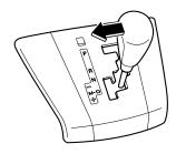
To return to automatic shift mode, shift the lever from M to D.
