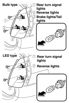
The LED-type bulbs for the brake lights/ taillights/Rear side-marker lights cannot be replaced by the customer. For bulb replacement, consult an Authorized Mazda Dealer.
