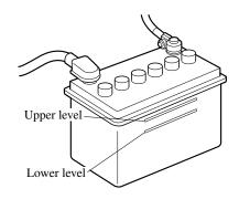
Inspect the electrolyte level at least once a week. If it's low, remove the caps and add enough distilled water to bring the level between the upper and lower level (illustration).
