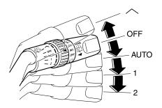
Turn the wipers on by pulling the lever down.
