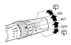
Turn the wiper on by turning the rear wiper/washer switch. **ON** — Normal **INT** — Intermittent
