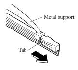
3. Remove the metal stiffeners from each blade rubber and install them in the new blade.
