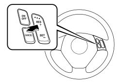
Your vehicle has a tap-up feature that allows you to increase your current speed in increments of 1.6 km/h (1 mph) by a momentary tap of the RES/+ button. Multiple taps will increase your vehicle speed 1.6 km/h (1 mph) for each tap.
