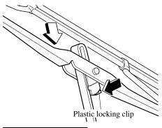
To prevent damage to the windshield let the wiper arm down easily, don't let it slap down on the windshield. 2. Hold the end of the rubber and pull until the tabs are free of the metal support.
