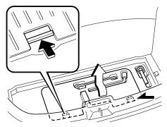
7. Remove the belt for securing the flat tire.
