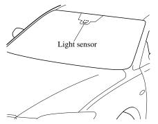
The light sensor also works as a rain sensor for the auto-wiper control. Keep hands and scrapers clear of the windshield when the ignition switch is in the ON position as fingers pinched or the wipers and wiper blades damaged when they activate automatically. If you are going to clean the windshield, be sure the wipers are turned off completely - this is particularly important when clearing ice and snow - when it is particularly tempting to leave the engine running.
