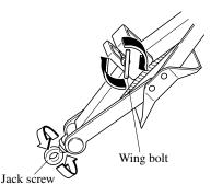
3. Turn the wing bolt completely to secure the jack.
