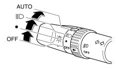
Turn the headlight switch to turn the headlights, other exterior lights and dashboard illumination on or off.
