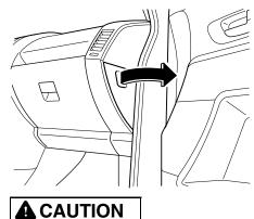
Pulling the cover off sideways may break the retaining tabs off.
