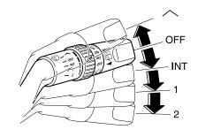
Turn the wipers on by pulling the lever down.
