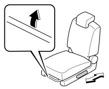
Make sure the lever returns to its original position and the seat is locked in place by attempting to push it forward and backward.
