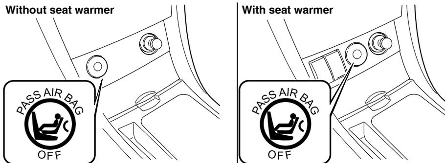
If the front passenger weight sensors are normal, the indicator light illuminates when the ignition switch is turned to the ON position. After about 6 seconds it goes out.
