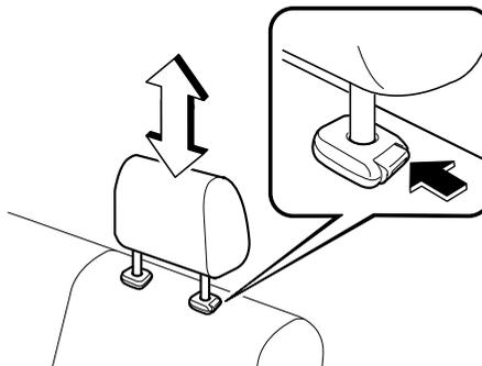
Adjust the head restraint so that the top is even with the top of the passenger's ears, never the passenger's neck.
