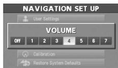
Select the appropriate button to set the volume to between **1** (minimum) and **7** (maximum).
