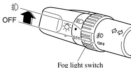
To turn the front fog lights off, rotate the fog light switch to the OFF position or turn the headlights off.
