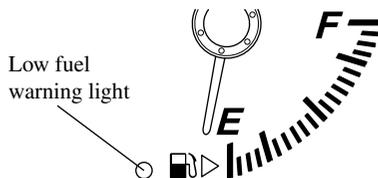
This warning light in the fuel gauge signals that the fuel tank will soon be empty. Refuel as soon as possible.
