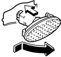
3. Install the new side turn signal unit in the reverse order of removal.
