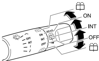
Turn the wiper on by turning the rear wiper/washer switch.
