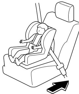
2. Secure the child-restraint system with the lap portion of the lap/shoulder belt. See the manufacturer's instructions on the child-restraint system for belt routing instructions.
