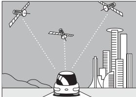
**GPS is a position detecting system utilizing the signals from GPS satellites deployed by the U.S. Department of Defense. The Mobile Navigation System uses input from three or more satellites and calculates the vehicle position based on the principle of triangulation. The positioning accuracy of the system corresponds to the error display of the GPS which is from about 30 to 200 meters.**
