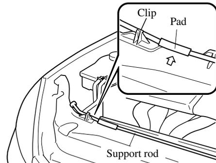
4. Secure the support rod in the stay hole indicated by the arrow to hold the hood open.
