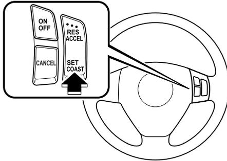
Your vehicle has a tap-down feature that allows you to decrease your current speed in decrements of 1.6 km/h (1 mph) by a momentary tap of the SET/COAST button. Multiple taps will decrease your vehicle speed 1.6 km/h (1 mph) for each tap.
