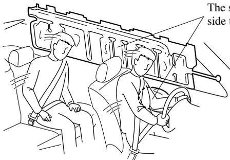
The side and curtain air bags will deploy only on the side the vehicle receives the force of the impact.
