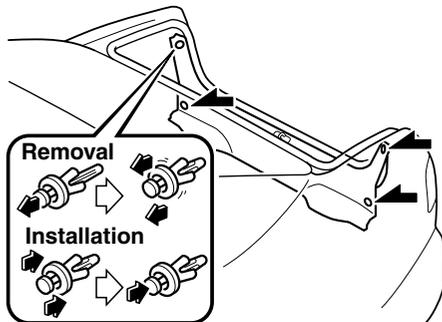
2. Pull the center of each plastic retainer and remove the retainers and partially open the trunk side trim.
