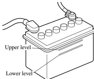
Inspect the electrolyte level at least once a week. If it's low, remove the cap and add enough distilled water to bring the level between the upper and lower level (illustration).
