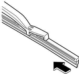
**▼ Replacing Rear Wiper Blade (5 Door)**
