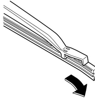
3. Remove the metal stiffeners from the blade rubber and install them in new blades.
