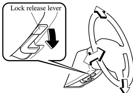
2. Tilt the steering wheel and/or adjust the steering column length to the desired positions, push the lever up to lock the column.
