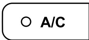
Push the A/C switch to turn the air conditioner on. The indicator light on the switch will illuminate when the fan control dial is set at position 1, 2, 3, or 4.
