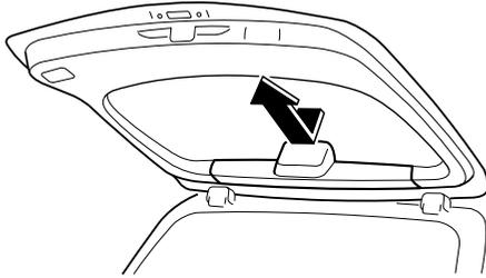
2. Disconnect the electrical connector from the socket.
