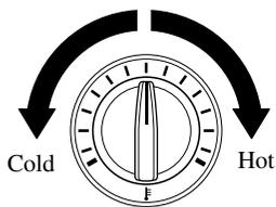
This dial controls temperature. Turn it clockwise for hot and counterclockwise for cold.
