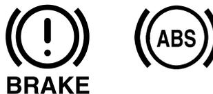
If the electronic brake force distribution control unit determines that some components are operating incorrectly, the control unit may turn the brake system warning light and the ABS warning light on at the same time. The problem is likely to be an electronic brake force distribution system.
