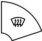
Press the switch to defrost the windshield and front door windows.
