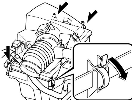
4. Lift off the air filter cover and remove the filter.
