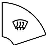
Press the windshield defroster switch. In this position, the
