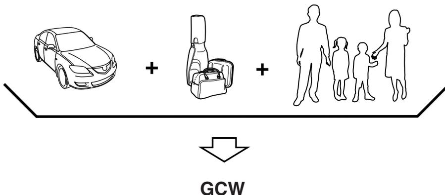
**GCW (Gross Combined Weight)** is the weight of the loaded vehicle (GVW) plus the weight of the fully loaded trailer.
