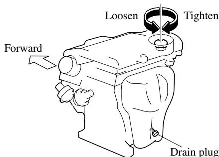
7. Start the engine and inspect around the drain plug for leaks.
