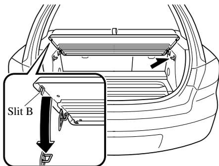
4. Rock the trunk board to make sure the board is installed securely.
