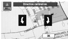
Use or to adjust the direction in which you are heading, and select **OK**.
