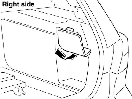
2. Turn the socket and bulb assembly counterclockwise and remove it.
