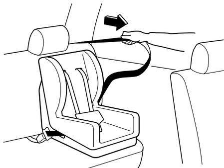
4. Push the child-restraint system firmly into the vehicle seat. Be sure the belt retracts as snugly as possible. Clicking from the retractor will be heard during retraction if the system is in the automatic locking mode. If the belt does not lock the seat down tight, repeat this step.
