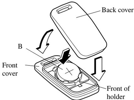
4. Align the front and back covers and snap the transmitter shut.
