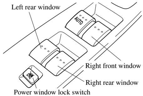
To open the window to the desired position, hold down the switch.
