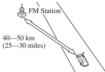
Signals from an FM transmitter are similar to beams of light because they do not bend around corners, but they do reflect. Unlike AM signals, FM signals cannot travel beyond the horizon. Therefore, FM stations cannot be received at the great distances possible with AM reception.
