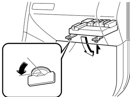
4. Locate the position of the suspected fuse by using the chart inside the fuse block cover.
