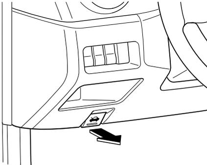
2. Slide the hood latch and lift the hood.
