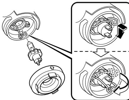
4. Swing the retaining spring out and away to free the headlight bulb.
