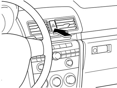
Depress the hazard warning flasher and all four turn signals will flash.
