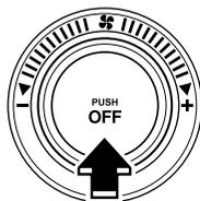
Pressing the OFF switch shuts off the climate control system.
