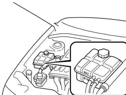
If it's at or near MIN, add enough coolant to the coolant reservoir to provide freezing and corrosion protection and to bring the level to MAX.
