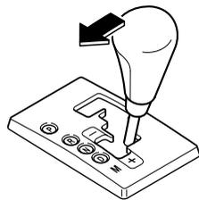
To return to automatic shift mode, shift the lever from M to D.
