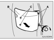
3. Turn the socket counterclockwise and remove it, and then remove the bulb from the socket by turning it counterclockwise while pressing in.
