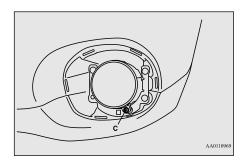
3. Turn the socket counterclockwise to remove it.
