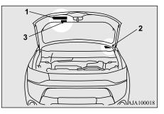
The air conditioning label is affixed on the inside panel of the engine hood.
