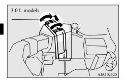
4. Replacing the air cleaner filter and put the cover back on in its original position.
