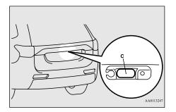
If the open switch is pressed while the power liftgate and all doors are unlocked, the power liftgate will open after the warning buzzer sounds 4 times and the hazard warning flasher blinks 2 times.
