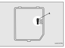
3. Clamp it on the fuse you wish to remove, and pull the fuse straight out from the fuse block.
