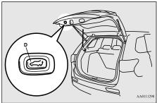
If the close switch on the power liftgate is pressed, the power liftgate will close after the warning buzzer sounds 3 times and the hazard warning flasher blinks 2 times. If the close switch is pressed once while the power liftgate is closing, the warning buzzer sounds once and the power liftgate opens.
