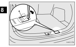
2. With the wheel nut wrench, loosen the tire hanger mounting bolt by turning it counterclockwise.
