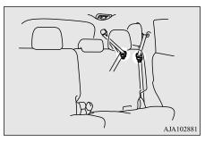
Put the seat belt webbing in the back slot (A) on the clip and insert the metal plate of the
