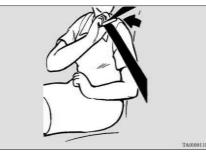
3. Pull the seat belt out slowly while holding the latch plate. Push the latch plate into the buckle until you hear a "click". Pull up on the belt to be sure the latch plate is locked securely in the buckle.
