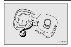
6. To re-install, turn the fuel tank filler pipe cap slowly clockwise until you hear clicking sounds, then gently push the fuel tank filler door closed.
