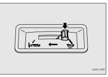
4. While lifting the seat belt buckle (A), gently lower the seat cushion. Make sure that there is a hook (B) at the position shown in the illustration.
