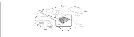
The camera for the rear view monitor system is located near the license plate. To adjust the image on the rear view monitor screen, press the setup button " on the left side of screen and select "Display" on the setup screen. Then select "Camera" to adjust the screen brightness and contrast.
