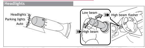
**Automatic light cut off system** Automatically turns lights off after 30-second delay, or lock switch on remote may be pushed afterlocking.
