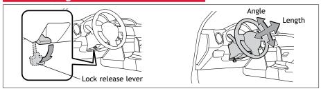
Hold wheel, push lever down, set angle and length, and return lever. NOTE: Do not attempt to adjust while the vehicle is in motion.
