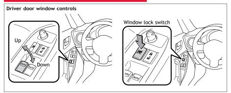
**Automatic operation** Push the switch completely down or pull it completely up and release to fully open. To stop window midway, lightly push the switch in the opposite direction.
