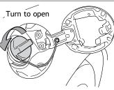
NOTE: Tighten until one click is heard. If the cap is not tightened enough, Check Engine "Kon" indicator may illuminate.
