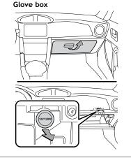
Designed for car accessories. Ignition switch must be in the "ACC" or "ON" position to be used.
