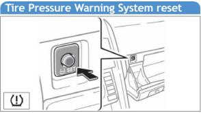
If tire pressure becomes critically low on any of the tires (excluding spare), indicator comes on. Pushing " 💬 SET" button should not turn off the light. Correctly adjusting tire inflation will turn off the light after a few minutes. After replacing/rotating tire or wheels, the system must be initialized.
