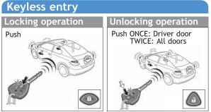
**NOTE:** After unlocking, if a door is not opened within thirty (30) seconds, all doors will relock for safety.
