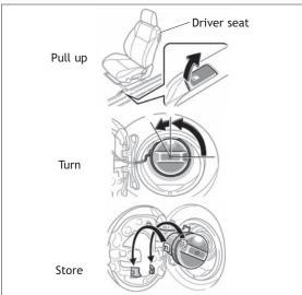
**NOTE:** Tighten cap until one click is heard. If the cap is not tightened enough, Check Engine "
