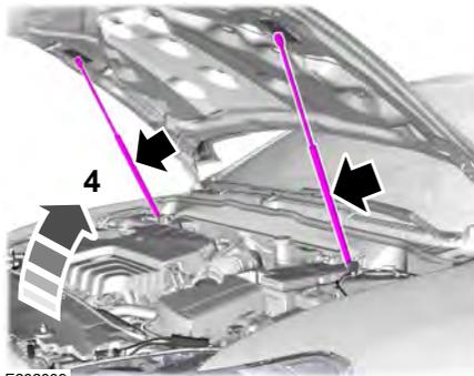
4. Open the hood. The hood struts automatically supports the hood.
