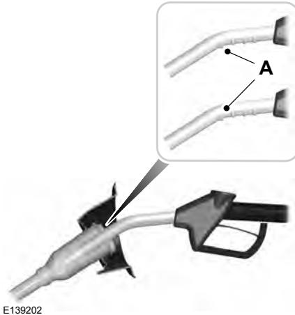
**Note:** When you insert the correct size fuel pump nozzle a spring loaded inhibitor opens.
