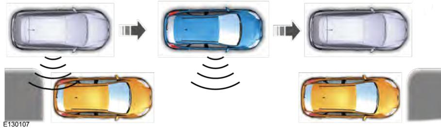
**Note:** You can also switch the system on after you have already driven partially or completely past a parking space. Press the Active Park Assist button and the system informs you if you have recently passed a suitable parking space.
