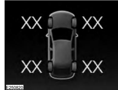
The tire pressure monitoring system measures pressure in your road tires and sends the tire pressure readings to your vehicle. You can view the tire pressure readings through the information display. See **General Information** (page 118). The low tire pressure warning light will turn on if the tire pressure is significantly low. Once the
