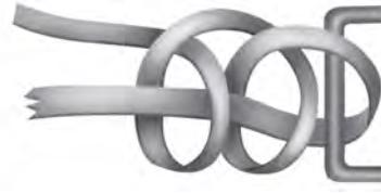
6. Secure the flat tire by tying a 2-half hitch knot.
