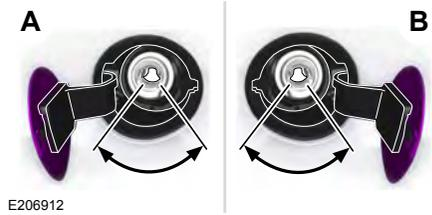
4. Operate the fuel pump nozzle within the area shown.
