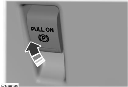
Pull the switch up to apply the electric parking brake.
