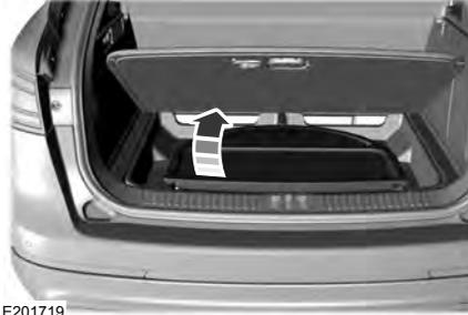
The high series has an additional cover that can be removed to access the spare tire or tire mobility kit.
