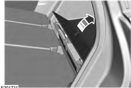
In-floor storage is located behind the second row of seats in the cargo area. Lift the strap to open.
