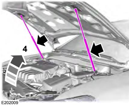
4. Open the hood. The hood struts automatically supports the hood.
