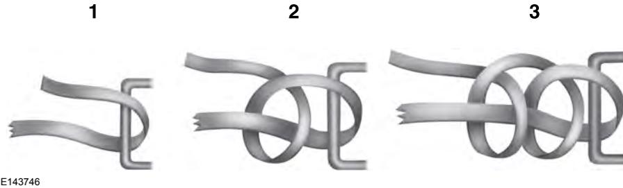
6. Secure the flat tire by tying a 2-half hitch knot.
