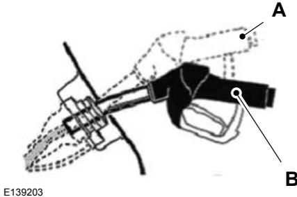
3. Hold the fuel pump nozzle in position B when refueling. Holding the fuel nozzle in position A can affect the flow of fuel and shut off the fuel nozzle before the fuel tank is full.
