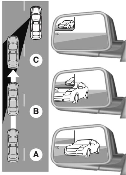
The approaching vehicle's image is small and near the inboard edge of the main mirror when it is at a distance. The image becomes larger and begins to move outboard across the main mirror as the vehicle approaches (A). Its image will transition from the main mirror and begin to appear in the blind spot mirror as the vehicle approaches (B). The vehicle will transition to your peripheral field of view as it leaves the blind spot mirror (C).
