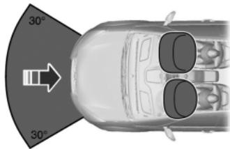
The driver and front passenger airbags will deploy during significant frontal and near frontal collisions.
