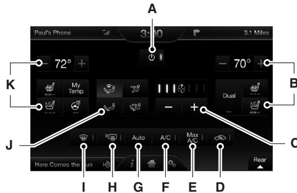
A. **Power:** Touch to turn the system on and off. Outside air cannot enter the vehicle when the system is off.
