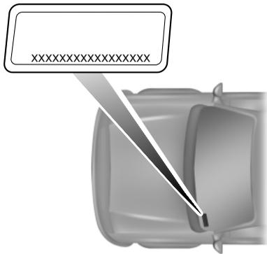
The vehicle identification number is located on the driver side instrument panel.
