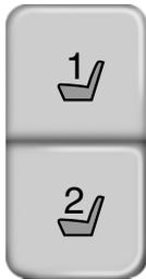
The memory control, located on the instrument panel, allows automatic positioning of the driver seat, power mirrors and power tilt/telescopic steering column (if equipped) to two programmable positions.
