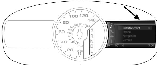
The infotainment display is located on the right side of your instrument cluster. It allows you to view and make minor adjustments to active modes without taking your hands off the wheel. For example:
