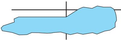
There is a distinct cut-off (change from light to dark) in the left portion of the beam pattern. The top edge of this cut-off should be positioned 2 inches (5 cm) below the horizontal reference line.
