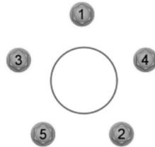
13. Remove the jack and fully tighten the lug nuts in the order shown. Refer to *Wheel lug nut torque specifications* later in this chapter for the proper lug nut torque specification.
