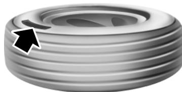
Tire Quality Grades apply to new pneumatic passenger car tires. The Quality grades can be found where applicable on the tire sidewall between tread shoulder and maximum section width. For example:
