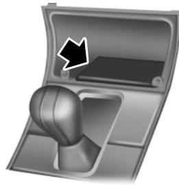
1. Using a screwdriver (or similar tool), carefully pry off and remove the Brake shift interlock access panel.
