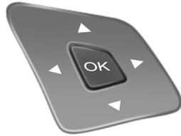
Use this control to adjust the right side of the cluster display. Navigate through the screen and press OK to select. Refer to the *MyLincoln Touch™* chapter.
