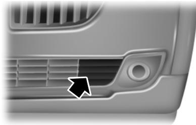
If a message regarding a blocked sensor appears in the information display, the radar signals from the sensor have been obstructed. The sensors are located behind a fascia cover near the driver side of the lower grille. When the sensors are obstructed, a vehicle ahead cannot be detected and the collision warning system does not function. The
