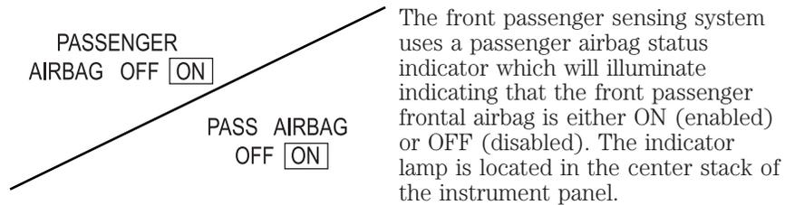
**Note:** The passenger airbag status indicator OFF and ON lamps will illuminate for a short period of time when the ignition is first turned on to confirm it is functional.
