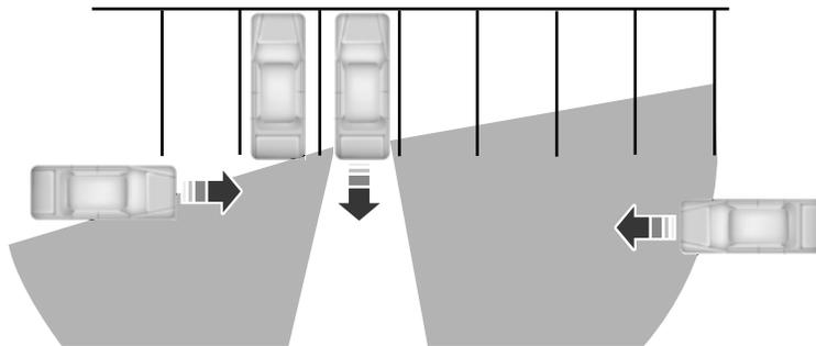
Zone coverage also decreases when parking at shallow angles. Here, the left sensor is mostly obstructed; zone coverage on that side is severely limited.
