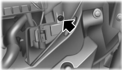
4. Locate the vertical adjuster on each headlamp. Using a Hex head driver, turn the adjuster either clockwise (to adjust down) or counterclockwise (to adjust up). The horizontal edge of the brighter light should touch the horizontal reference line.
