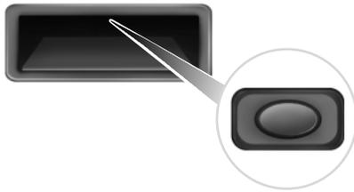
**To open the liftgate:** Press the button located in the top of the liftgate pull cup handle to unlatch the liftgate, then pull on the outside handle.
