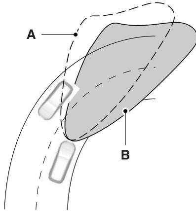
**Note:** The system has a power-up movement check feature. When the vehicle is started, the lamps track left to right, then back to center to alert the driver that the system is working properly. There is a delay of two to five seconds before the adaptive headlamp system will operate when the vehicle is driven, as the system is inactive below 3 mph (5 km/h).
