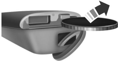
2. Twist a thin coin in the slot hidden behind the backup key slot to remove the battery cover.
