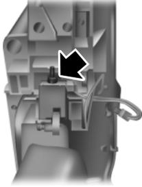
2. Locate the brake shift interlock lever in front of the shifter assembly.
