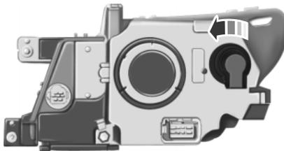
4. Rotate the bulb socket counterclockwise and remove from the lamp assembly.
