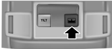
Press and release the control to open the sunshade. The front and rear sunshades open simultaneously.
