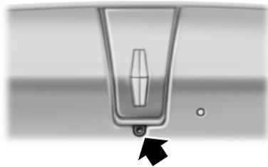
The camera is located on the liftgate.
