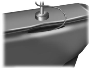
When in use, the rear outboard safety belts can be used with the comfort guides. This guide is attached to the head restraint and is stored in a pocket in the seatback.
