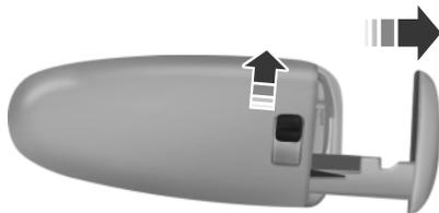
The intelligent access key also contains a removable mechanical key blade that can be used to unlock the driver door. Slide the release on the back of the transmitter to release the mechanical key blade, then pull the blade out.
