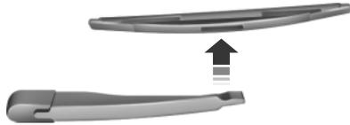
4. Attach the new wiper to the wiper arm and press it into place until a click is heard.
