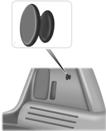
The utility hook can be used to hang small items such as grocery bags, etc. Do not hang more than 10 pounds (4.5 kilograms) on the hook.
