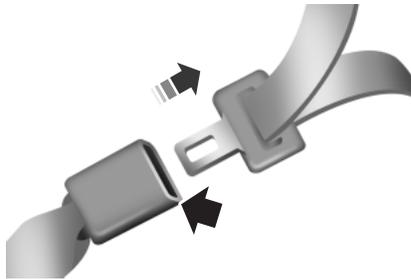
2. To unfasten, press the release button and remove the tongue from the buckle.
