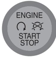
To turn the ignition on, press the start button once. It is located on the instrument panel to the right of the steering wheel. All electrical circuits and accessories are operational, and warning lamps and indicators will illuminate.
