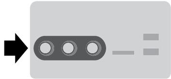
Your A/V inputs allow you to connect an auxiliary audio/video source (game systems, personal camcorders, etc.) by connecting RCA cords (not included) to these input jacks. The jacks are yellow, red and white and are located either
