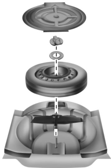
3. Lift the carpeted load floor panel located in the rear of the vehicle and remove the spare tire cover (if equipped).
