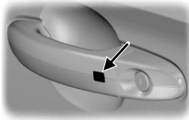
Press and hold the door handle lock sensor to lock the vehicle.
