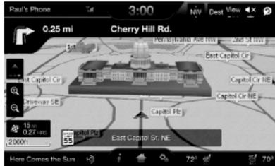
Change the appearance of the map display by repeatedly pressing the arrow button in the upper left corner of the screen. It toggles between three different map modes; Heading up, North up, and 3D.
