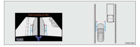
Example 2: When parking on the shoulder Approach the shoulder, but do not allow the vehicle width line to overlap the curb or other obstacles. After confirming the distance to the shoulder of the road, maneuvering the vehicle so that the vehicle width line and the curb or other obstacle are parallel allows the vehicle to
