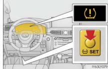
When position of each tire is determined, the inflation pressure of each tire will be displayed on the multi-information display.
