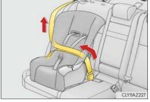
6 If the child restraint has a top tether strap, the top tether strap should be latched onto the top tether strap anchor.  $(\rightarrow P. 64)$
