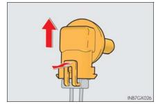
A Replace the light bulb, and install the bulb base.
