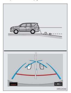
When any part of the vehicle sags due to the number of passengers or the distribution of the load, there is a margin of error between the guide lines on the screen and the actual distance/course on the road.
