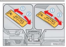
The seat heaters and ventilators can be used when the engine  $\overline{\text{switch}}$  is in IGNITION ON mode.
