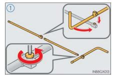
Assemble the jack handle extension bar and the jack handle and tighten the bolt and the screw.
