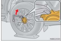
3 Slightly loosen the wheel nuts (one turn).
