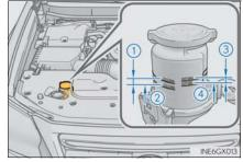
Hot: The vehicles has been driven around 50 mph (80 km/h) for 20 minutes, or slightly longer in frigid temperatures.
