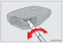
Remove the depleted battery.
