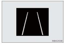
When solid lane lines are shown: The LDA system is active.
