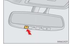
If the garage door opener motor activates when the HomeLink button is pressed, the garage door opener motor recognizes the HomeLink signal.
