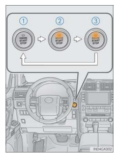
If the engine is stopped with the shift lever in a position other than P, the engine switch will not be turned off but instead be turned to ACCESSORY mode. Perform the following procedure to turn the switch off:
