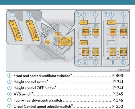
Crawl Control ON/OFF switch\*
