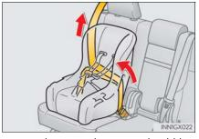
If the child restraint has a top tether strap, the top tether strap should be latched onto the top tether strap anchor.  $(\rightarrow P. 67)$
