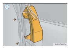
2 Close the back door half way and remove the lamp assembly.
