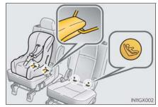
Seat belts equipped with a child restraint locking mechanism (ALR/ ELR belts except driver's seat belt)  $(\rightarrow P.32)$
