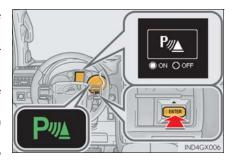
When the sensors detect an obstacle, a graphic is shown on the multi-information display, multimedia screen (if equipped) and navigation system screen (if equipped) depending on the position and distance to the obstacle.
