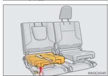
3 Pull the seatback lock release lever and fold the seatback down.
