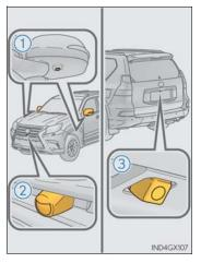
If dirt or foreign matter (such as water droplets, snow, mud etc.) is adhering to the camera, it cannot transmit a clear image. In this case, flush it with a large quantity of water and wipe the camera lens clean with a soft and wet cloth.
