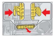
Femove the air conditioning filter from the filter case and replace it with a new one.
