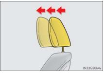
The position of the head restraint can be adjusted forward in 4 stages.
