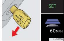
If the lever is operated while the vehicle speed is below approximately 30 mph (50 km/h) and a preceding vehicle is present, the set speed will be adjusted to approximately 30 mph (50 km/h).
