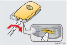
**3** Remove the depleted battery.
