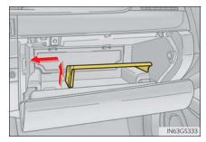
3 Press the tabs and remove the filter cover.
