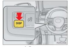
2 Press the "DISP" button to switch between on and off.
