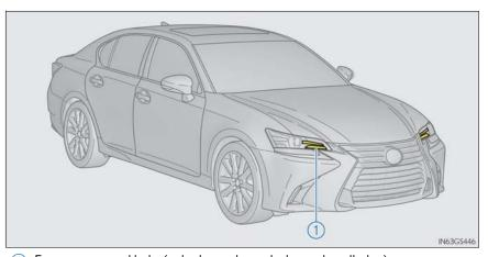
1 Front turn signal light (vehicles with single-beam headlights)
