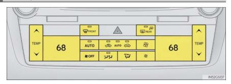
Press " $\wedge$ " on  $\left| \begin{array}{c} \bullet \end{array} \right|$  to increase the temperature and " $\vee$ " to decrease the tem-
