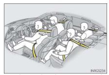
The pretensioner does not activate in the event of a minor frontal impact, a minor side impact, a rear impact or a vehicle rollover.
