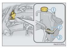
If the level is on or below the "LOW" line, add coolant up to the "FULL" line. ( $\rightarrow$ P. 512)
