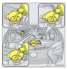
**6** Start the engine and turn the air conditioning system on to check that the radiator cooling fans operate and to check for coolant leaks from the radiator or hoses.
