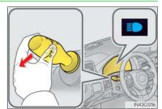
2 Press the Automatic High Beam switch.
