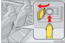
Connect by inserting the bottle straight into the compressor, and make sure that the protruding part of the bottle is properly aligned with the groove in the case.
