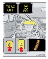
■ When the message is displayed on the multi-information display showing that TRAC has been disabled even if 👼 has not been pressed (GS350/GS300)
