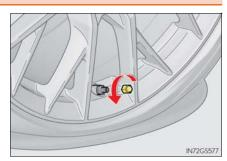
2 Remove the air release cap from the hose.
