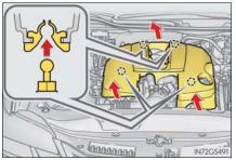
Raise the front of the engine cover to remove the front clips, and then raise the rear of the engine cover to remove the rear clips.
