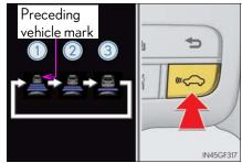
Pressing the switch changes the vehicle-to-vehicle distance as follows:
