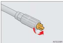
3 Connect the hose to the valve. Screw the end of the hose clockwise as far as possible.
