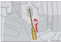
Manual operation of the parking brake The parking brake cannot be set manually.
