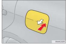
Turn the fuel tank cap slowly to remove it and put it into the holder on the fuel filler door.
