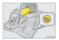
Seat belts equipped with a child restraint locking mechanism (ALR/ ELR belts except driver's seat belt)  $(\rightarrow P.37)$
