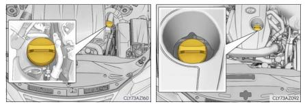
Make sure to check the oil type and prepare the items needed before adding oil.
