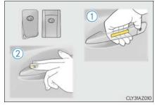
② Touch the lock sensor (indentation on the upper part of the front door handle) to lock all the doors.
