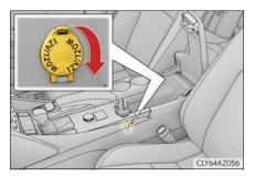
The power outlet can be used when the engine switch is in  $\mathsf{ACCESSORY}$  or <code>IGNITION</code> ON mode.
