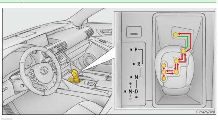
While the engine switch is in IGNITION ON mode, move the shift lever with the brake pedal depressed.
