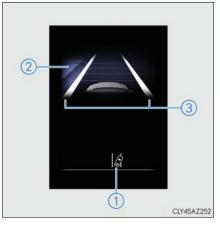
Indicates that steering wheel assistance of the steering control function is operating.
