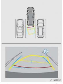
**4** Once the vehicle width guide lines and the parking space lines are parallel, straighten the steering wheel and back up slowly until the vehicle has completely entered the parking space.
