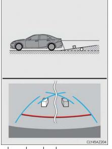
• When the ground behind the vehicle slopes up sharply
