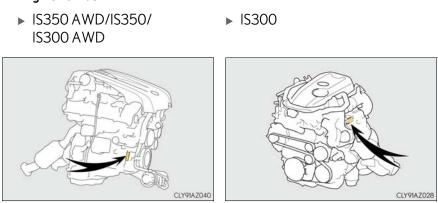
The engine number is stamped on the engine block as shown.
