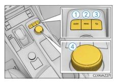
Move the controller to display the left or right side of the screen.
