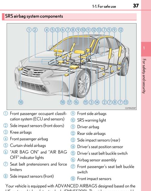
US motor vehicle is equipped with ADVANCED AIRBAGS designed based on the US motor vehicle safety standards (FMVSS208). The airbag sensor assembly (ECU) controls airbag deployment based on information obtained from the sensors etc. shown in the system components diagram above. This information includes crash severity and occupant information. As the airbags deploy, a chemical reaction in the inflators quickly fills the airbags with non-toxic gas to help restrain the motion of the occupants.
