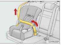
**6** If the child restraint has a top tether strap, the top tether strap should be latched onto the top tether strap anchor. ( $\rightarrow$ P. 64)
