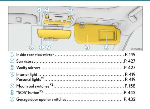
\*1: The illustration shows the front, but they are also equipped in the rear. \*2: If equipped
