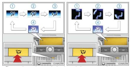
The air outlets used are switched each time the button is pressed.
