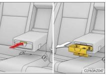
To open, pull down the armrest and press the button and release the rear cup holder on the armrest.
