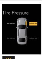
Indicates a malfunction in the tire pressure warning system
