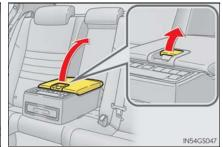
Pull up the lever to release the lock and lift the lid.
