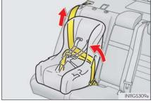
6 If the child restraint has a top tether strap, the top tether strap should be latched onto the top tether strap anchor.  $(\rightarrow P. 62)$
