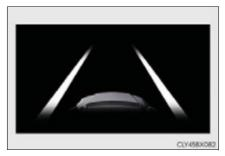
Indicates that the system is recognizing white (yellow) lines. When the vehicle departs from its lane, the white line displayed on the side the vehicle departs from flashes amber.
