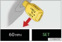
The vehicle speed at the moment the lever is released becomes the set speed.
