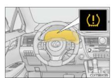
When position of each tire is determined, the inflation pressure of each tire will be displayed on the multi-information display.
