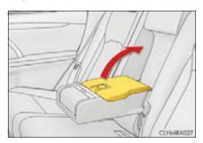
Pull up the lever to release the lock, and lift the lid.
