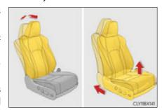
If the head restraint cannot be removed, raise it to the uppermost position.
