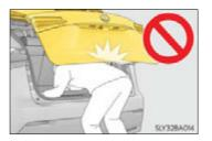
Vehicles with a power back door: The back door may suddenly shut if it is not opened fully, while on a steep incline.
