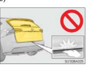
Use caution when using the back door closer as it still operates when the power back door system is canceled.
