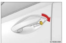
3 Remove the key, return the handle, and then pull the handle again.
