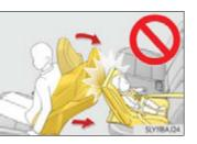
• Do not allow the child to lean his/her head or any part of his/her body against the door or the area of the seat, rear pillars or roof side rails from which the SRS curtain shield airbag deploys even if the child is seated in the child restraint system. It is dangerous if the SRS curtain shield airbag inflates, and the impact could cause death or serious injury to the child.
