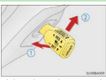
However, resuming is available when the vehicle speed is more than approximately  $25~{\rm mph}$  (40 km/h).
