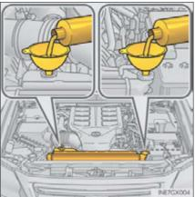
Start the engine and turn the air conditioning system on to check that the radiator cooling fans operate and to check for coolant leaks from the radiator or hoses.
