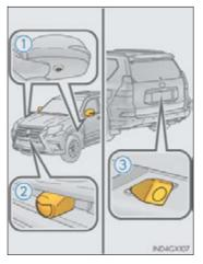
If the camera lens becomes dirty, it cannot transmit a clear image. If water droplets, snow or mud adhere to the lens, rinse with water and wipe with a soft cloth. If the lens is extremely dirty, wash it with a mild cleanser and rinse.
