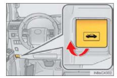
2 Move the auxiliary catch lever to side direction and lift the hood.
