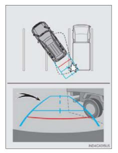
Visually check the surroundings and the area behind the vehicle. On the screen, it appears that a truck is parking at point ②. However, in reality if you back up to point ①, you will hit the truck. On the screen, it appears that ① is closest and ③ is farthest away. However, in reality, the distance to ① and ③ is the same, and ② is farther than ① and ③.
