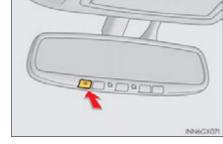
If the garage door opener motor activates when the HomeLink button is pressed, the garage door opener motor recognizes the HomeLink  $^{\circledR}$  signal.
