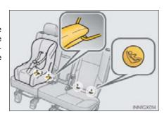
Seat belts equipped with a child restraint locking mechanism (ALR/ ELR belts except driver's seat belt)  $(\rightarrow P.30)$
