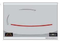
Screen display and beep sounds provide an estimation of the point at which you should turn the steering wheel when parallel parking. If the position the vehicle is to be parked in is narrower than usual, narrow mode can be used.
