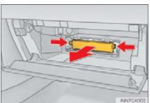
4 Slide and pull out the filter. Replace the filter with a new one.
