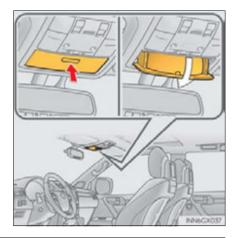
To use the overhead console when the conversation mirror is open, further extend the lid.  $(\rightarrow P.404)$
