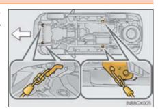
If you use cables or chains to tie down your vehicle, the angles shaded in black must be  $45^{\circ}$ .
