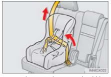
If the child restraint has a top tether strap, the top tether strap should be latched onto the top tether strap anchor.  $(\rightarrow P. 64)$
