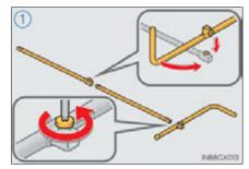
② Assemble the jack handle extension bar and the jack handle and tighten the bolt and the screw.
