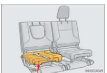
3 Pull the seatback lock release lever and fold the seatback down.
