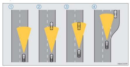
The vehicle travels at the speed set by the driver. The desired vehicle-to-vehicle distance can also be set by operating the vehicle-to-vehicle distance control.
