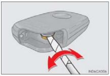
Remove the depleted battery.
