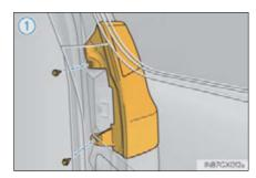
Close the back door half way and remove the lamp assembly.
