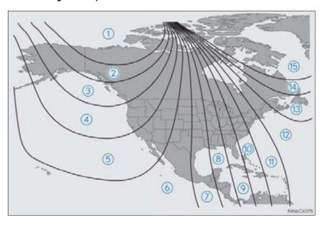
The direction display deviates from the true direction determined by the earth's magnetic field. The amount of deviation varies according to the geographic position of the vehicle.
