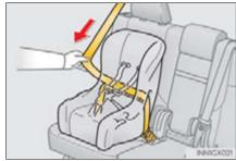
S While pushing the child restraint system into the seat, allow the shoulder belt to retract until the child restraint system is securely in place.
