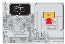
When vehicle speed exceeds 18 mph (30 km/h), the rear height control air suspension turns on automatically.
