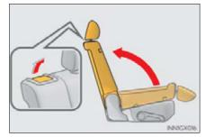
2 Place the child restraint system on the seat facing the rear of the vehicle.
