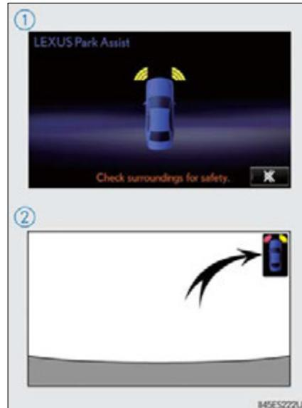
**Sensor detection display, obstacle distance**
