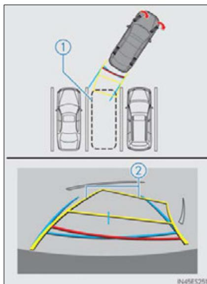
3 When the rear position of the vehicle has entered the parking space, turn the steering wheel so that the vehicle width guide lines are within the left and right dividing lines of the parking space.
