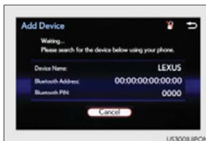
A PIN code are not required for SSP (Secure Simple Pairing) compatible Bluetooth® devices. Depending on the device, you may need to select Yes to register, or No to cancel on the device.
