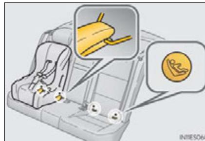
Seat belts equipped with a child restraint locking mechanism (ALR/ELR belts except driver's seat belt) (→P.33)
