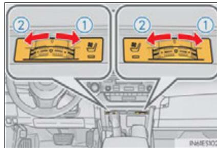
The seat heaters and ventilators can be used when the power switch is in ON mode.
