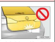
• Do not pull on the back door damper stay to close the back door, and do not hang on the back door damper stay.
