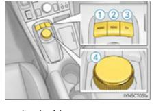
Move the controller to display the left or right side of the screen.
