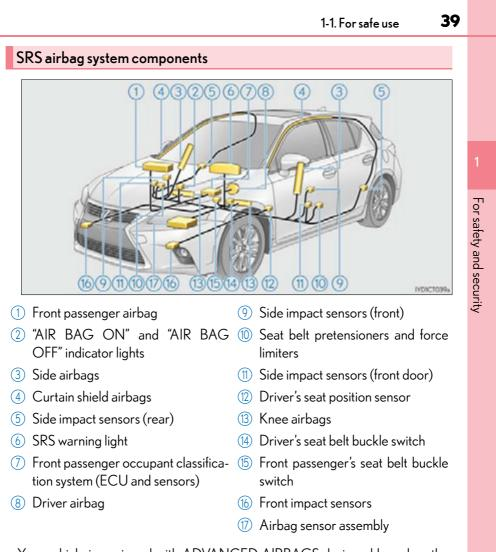
Your vehicle is equipped with ADVANCED AIRBAGS designed based on the US motor vehicle safety standards (FMVSS208). The airbag sensor assembly (ECU) controls airbag deployment based on information obtained from the sensors etc. shown in the system components diagram above. This information includes crash severity and occupant information. As the airbags deploy, a chemical reaction in the inflators quickly fills the airbags with non-toxic gas to help restrain the motion of the occupants.
