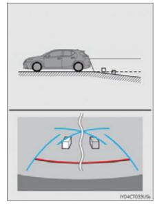
• When any part of the vehicle sags When any part of the vehicle sags due to the number of passengers or the distribution of the load, there is a margin of error between the guide lines on the screen and the actual distance/course on the road.
