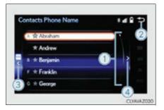
④ Indicator turns on when you can move the controller right to view additional screen text.
