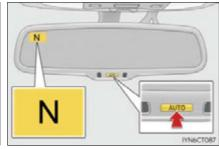
To turn the compass on or off, press the "AUTO" button for more than 3 seconds.
