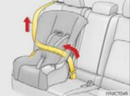
**5** If the child restraint has a top tether strap, the top tether strap should be latched onto the top tether strap anchor.  $(\rightarrow P. 61)$
