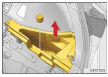
**4** Remove the 12-volt battery maintenance cover.
