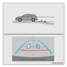
• When any part of the vehicle sags When any part of the vehicle sags due to the number of passengers or the distribution of the load, there is a margin of error between the fixation guide lines on the screen and the actual distance/ course on the road.
