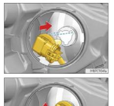
6 When installing the cover, conduct step 1 in reverse.
