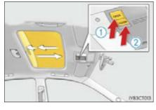
$^{\star}$ : Lightly press either end of the moon roof switch to stop the moon roof partway.
