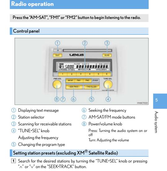
**2** Press and hold the button (from the "1" button to the "6" button) the station is to be set to until you hear a beep.
