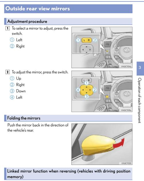
When the mirror select switch is in the "L" or "R" position, the outside rear view mirrors will automatically angle downwards when the vehicle is reversing in order to give a better view of the ground.
