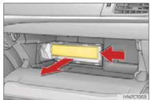
**5** Slide and pull out the filter. Replace it with a new one.
