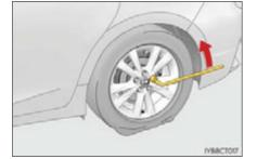
**3** Turn the tire jack portion (A) by hand until the notch of the jack is in contact with the jack point.
