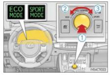
When the driving mode select switch is turned left, the "ECO MODE" indicator comes on in the instrument cluster.
