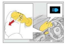
**2** Press the Automatic High Beam switch.
