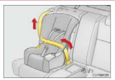
After installing the child restraint system, rock it back and forth to ensure that it is installed securely.
