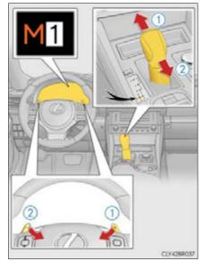
When in the M position, the gear will not change unless the shift lever or paddle shift switches are operated.
