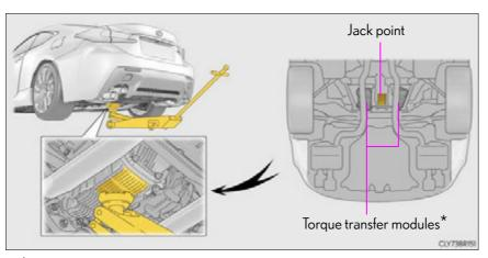
$<sup>\</sup>ensuremath{^\star}$  : Do not place the floor jack under either torque transfer module.
