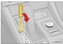
**5** Press the shift lock override button. The shift lever can be shifted while the button is pressed.
