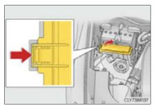
ightharpoonup Engine compartment: type B fuse box
