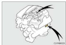
The engine number is located as shown.
