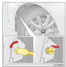
2 Disengage the fender liner from the clamp then pull it back.
