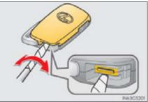
**3** Remove the depleted battery.
