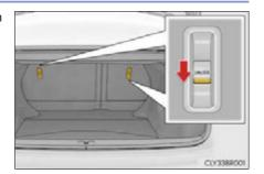
2 Pull the seatback lock release lever and fold the seatback down.
