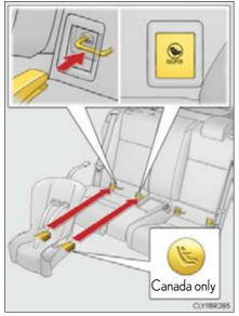
3 After installing the child restraint system, rock it back and forth to ensure that it is installed securely.
