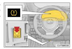
Wait for a few minutes with the engine switch in IGNITION ON mode and then turn the engine switch off.
