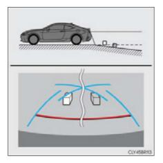
• When any part of the vehicle sags When any part of the vehicle sags due to the number of passengers or the distribution of the load, there is a margin of error between the guide lines on the screen and the actual distance/course on the road.
