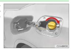
2 Close the fuel filler door, and press the center of the rear edge of the fuel filler door until you hear a click. When you lock the doors, the fuel filler door will also lock.
