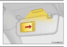
If the vanity lights remain on when the engine switch is turned off, the lights will go off automatically after 20 minutes.
