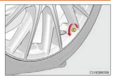
**2** Extend the hose. Remove the air release cap from the hose.
