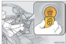
3 Press the engine switch within 10 seconds of the buzzer sounding, keeping the brake pedal depressed.
