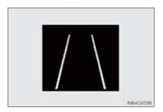
When solid lane lines are shown: The LDA system is active.
