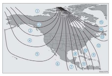
The direction display deviates from the true direction determined by the earth's magnetic field. The amount of deviation varies according to the geographic position of the vehicle.
