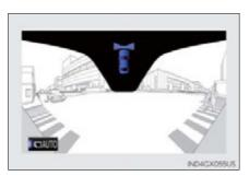
The image from the side camera is displayed. Use this monitor to help check the area to the right of the vehicle, for example when taking off and stopping, when turning right, etc. If displayed, the course line can be used as rough guide for steering wheel operation when turning right.  $(\rightarrow P. 288)$
