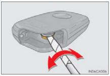
Remove the depleted battery.
