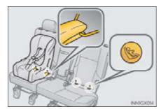
Seat belts equipped with a child restraint locking mechanism (ALR/ ELR belts except driver's seat belt)  $(\rightarrow P.30)$
