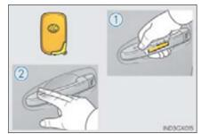
2 Touch the lock sensor (the indentation on the upper part or lower part of the front door handle) to lock the doors.
