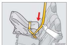
S While pushing the child restraint system down into the seat, allow the shoulder belt to retract until the child restraint system is securely in place.
