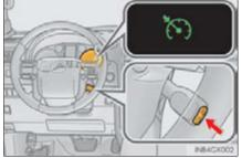
2 Accelerate or decelerate the vehicle to the desired speed, and push the lever down to set the speed.
