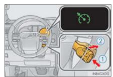
When in constant speed control mode, to return to vehicle-to-vehicle distance control mode, push the lever forward again and hold for approximately 1 second.
