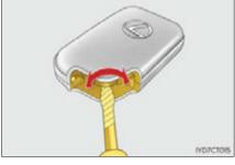
Remove the depleted battery.
