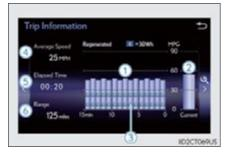
Average fuel consumption for the past 15 minutes is divided by color into past averages and averages attained since the power switch was last turned to ON mode. Use the displayed average fuel consumption as a reference.
