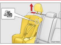
2 Open the anchor bracket cover, latch the hook onto the anchor bracket and tighten the top tether strap.
